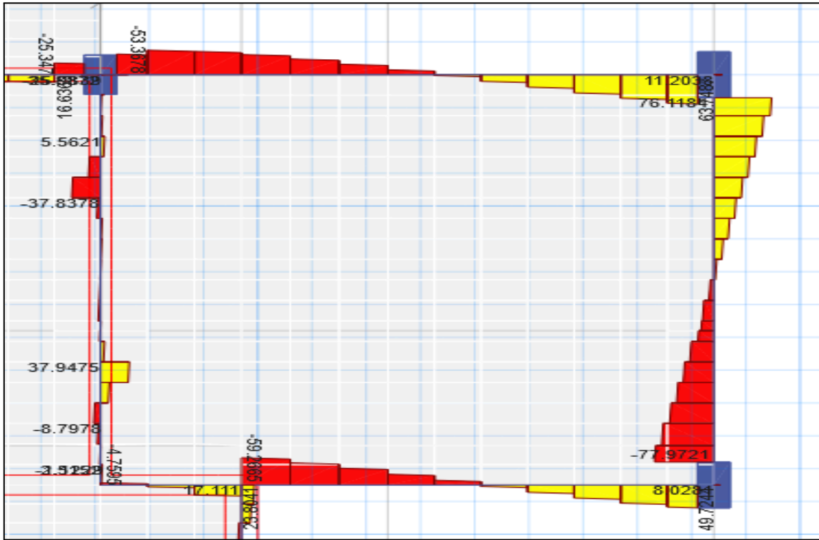
Figure 3.34: Shear forces in column-supported beams
