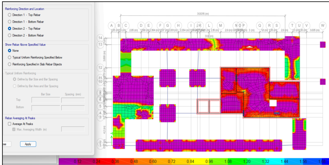
Figure 3.78: Top rebar reinforcing direction 2
