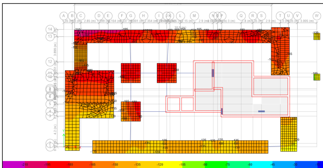
Figure 6.7: Contour map of soil pressure in footings for the determinant load combination (ETABS Output)
