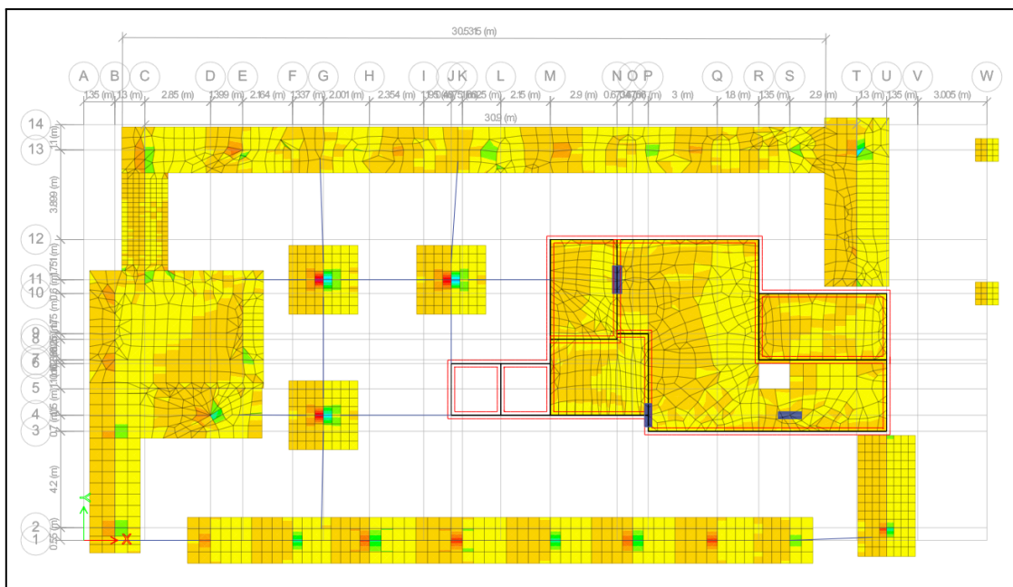
Figure 6.9: Contour map of shear force V13 in footings for the ENVELOPE load combination
