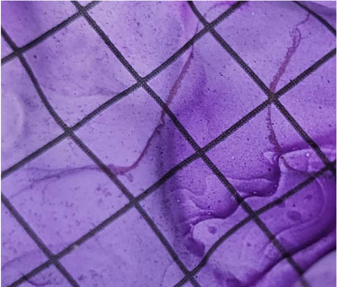
Figure C 1: Filter membrane after Nile Red dye staining for sample 1
