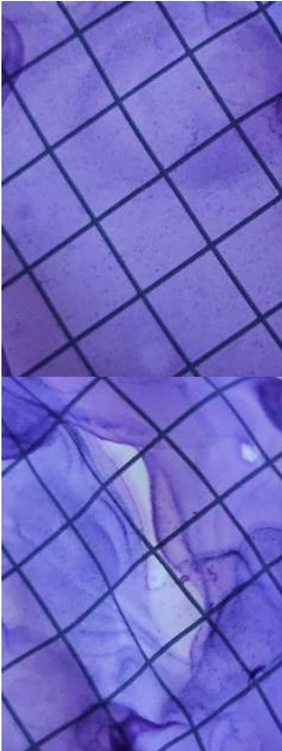
Figure C 3: Filter membrane after Nile Red dye staining for sample 3
