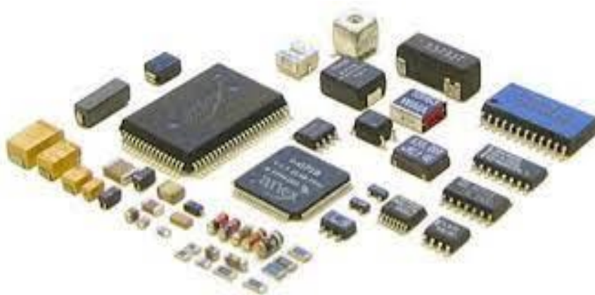
Figure (6) 2.4. :Types of SMD Components
