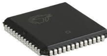
Figure (10) 2.8. : Surface Mount QFJ (PLCC)
