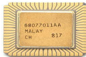
Figure (11) 2.9. : Leadless ceramic chip carriers (LCCC)
