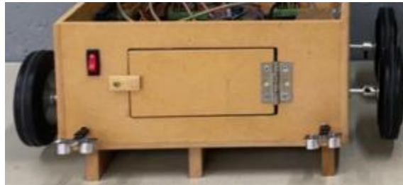
Figure 3-3 Main On/Off switch ( external view ) and placement on the base
