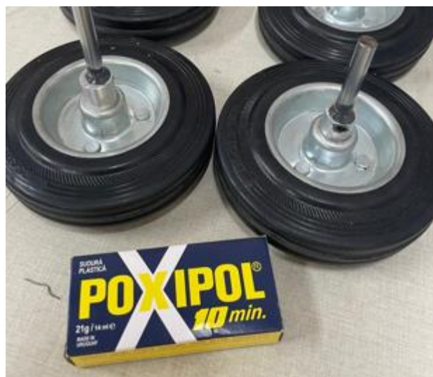
Figure 5-1 Wheel hub and coupler secured using Poxipol to prevent loosening under load
