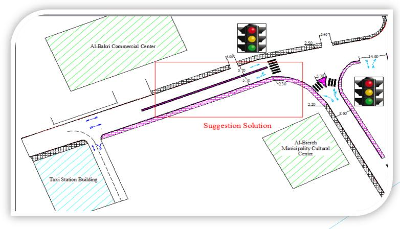
The second problem is Busses Station movements inside the intersection and presence of busses that make a conflicting points when enter and exit the station.
