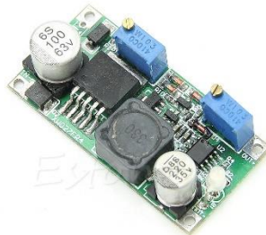
Figure 12: Buck-Boost Converter Module
