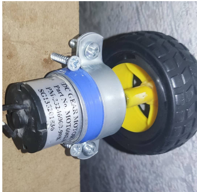
Figure 12: DC low speed geared motor
