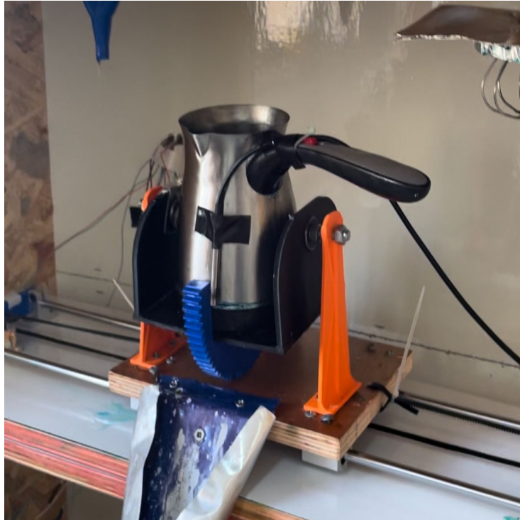
Figure 4.12: Heater moving system along the production line
