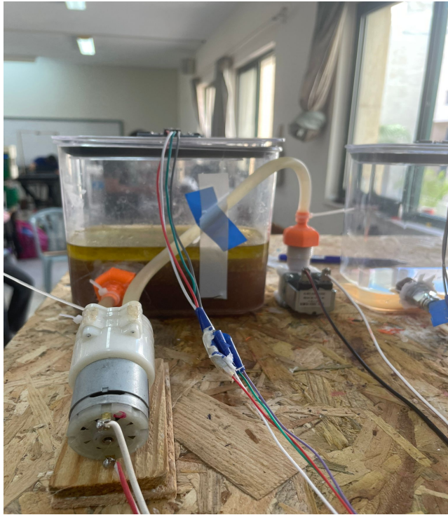
Figure 4.6: Pumping for oil , water and soda
