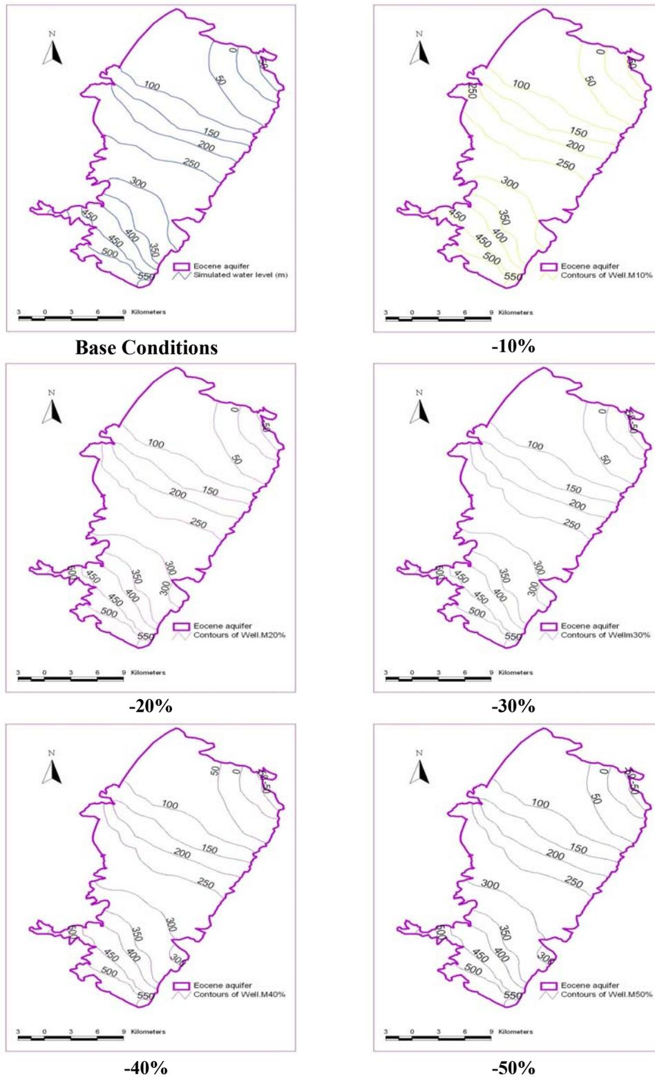
**Figure 7.28:** The Contours of Water Table Elevation for Different Decrease Percentages in Pumping Rates
