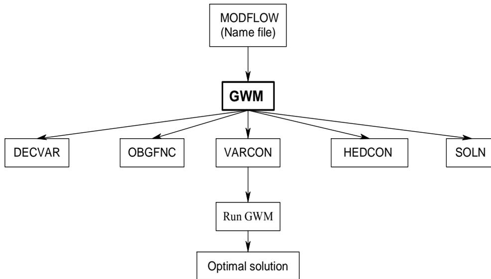
**Figure 8.4:** The Files Utilized in Developing the GWM for the Optimal Management of the Eocene Aquifer
