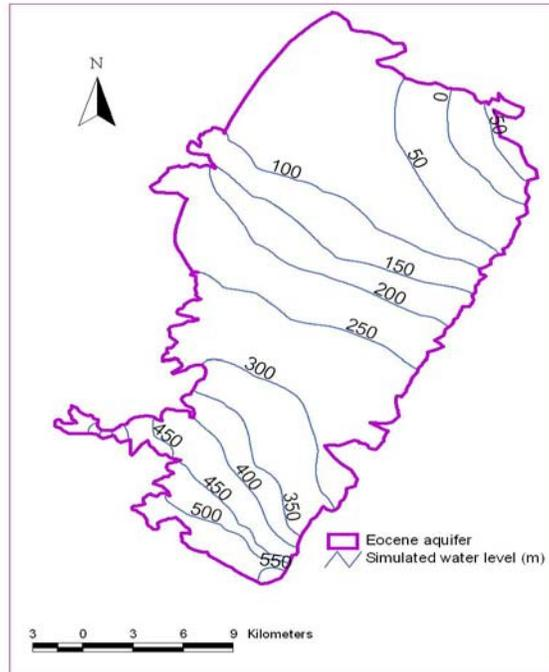
**Figure 7.13:** The Contours of the Simulated Water Table Elevations of the Eocene Aquifer
