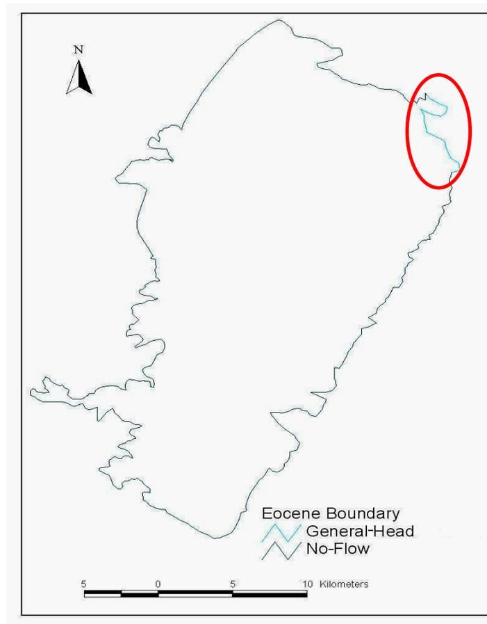
**Figure 7.2:** Boundary Conditions for the Eocene Aquifer
