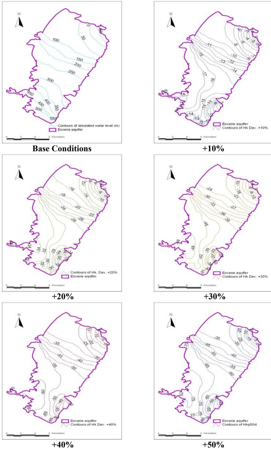
**Figure 7.17:** The Contours of Water Table Deviation for Different Increase Percentages in the Hydraulic Conductivity Values
