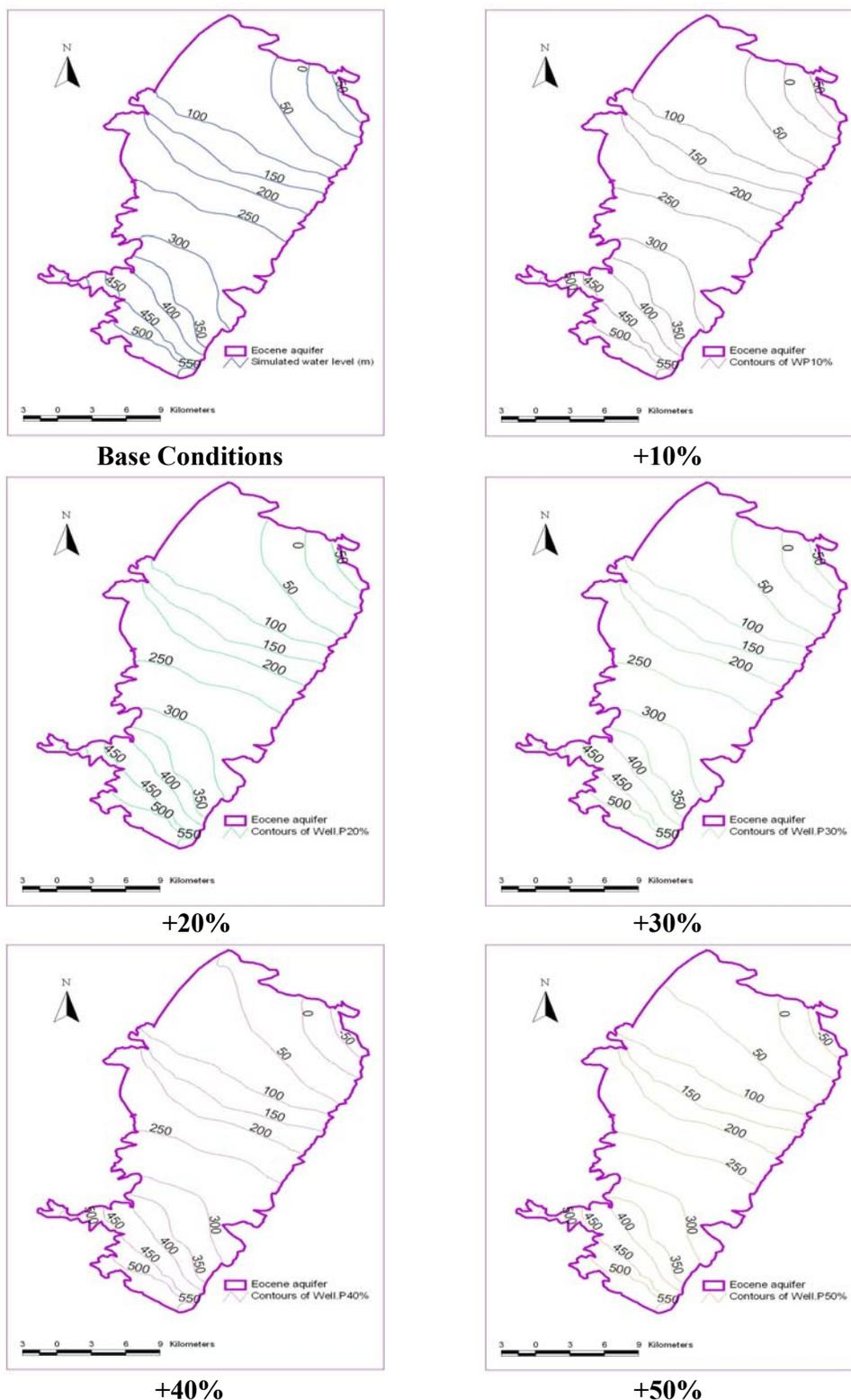
**Figure 7.27:** The Contours of Water Table Elevation for Different Increase Percentages in Pumping Rates
