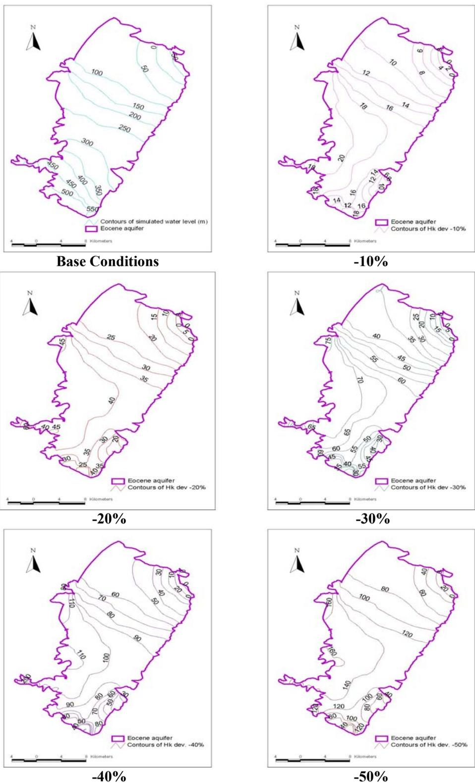
**Figure 7.18:** The Contours of Water Table Deviation for Different Decrease Percentages in the Hydraulic Conductivity Values
