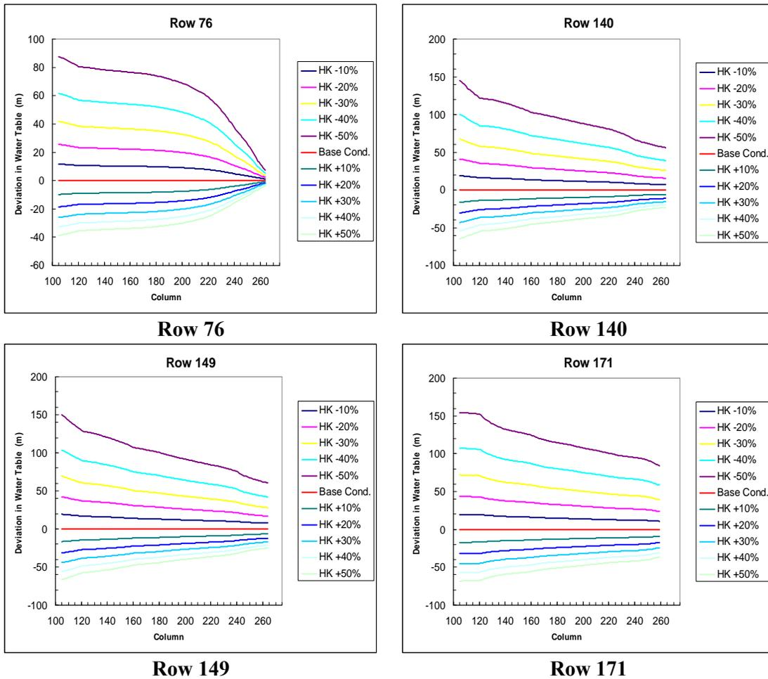
**Figure 7.19:** Deviation in Water Table Elevation for Specific Row and Columns to Perturbations in the Hydraulic Conductivity
