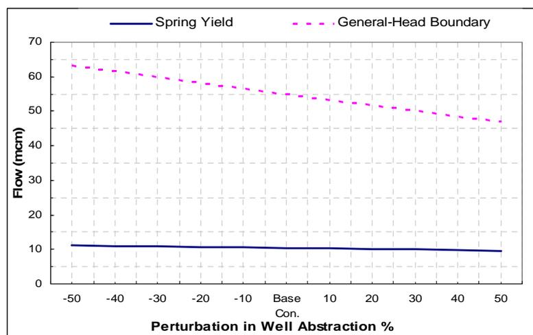
**Figure 7.32:** Sensitivity in Spring Yield and General-Head Boundary Outflow Due to Perturbations in Pumping Rates
