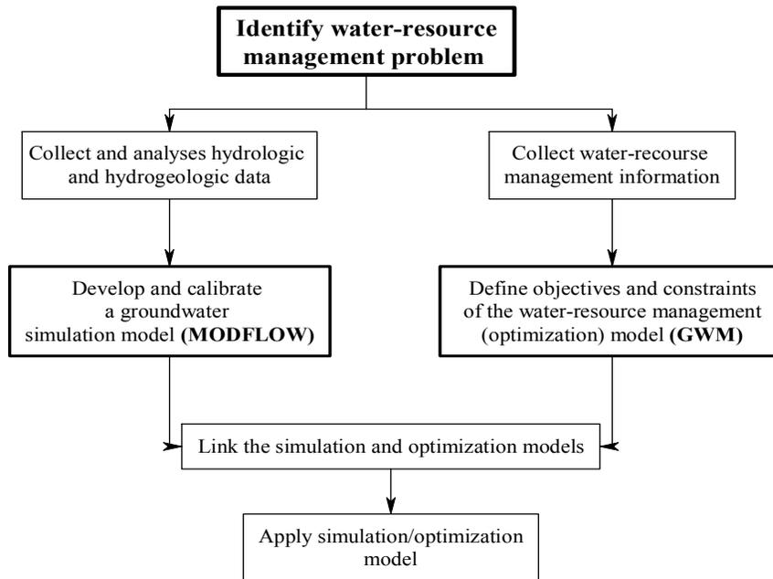
**Figure 8.1:** The Steps for the Development and Application of a Groundwater Simulation/Optimization Model for the Eocene Aquifer
