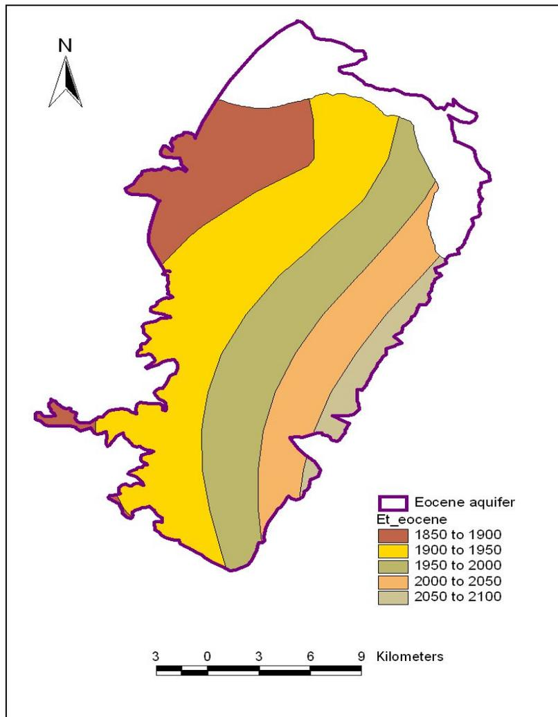
**Figure 2.7:** Evaporation Rates of the Eocene Aquifer. (Note that for Areas Outside the West Bank no Data is Available)
