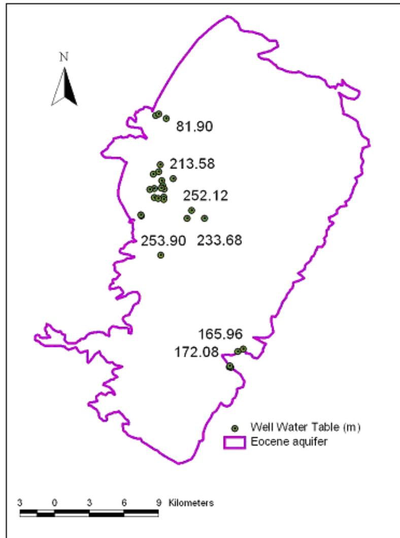
**Figure 7.9:** Water Table Elevations for Selected Wells in the Eocene Aquifer for Year 2003
