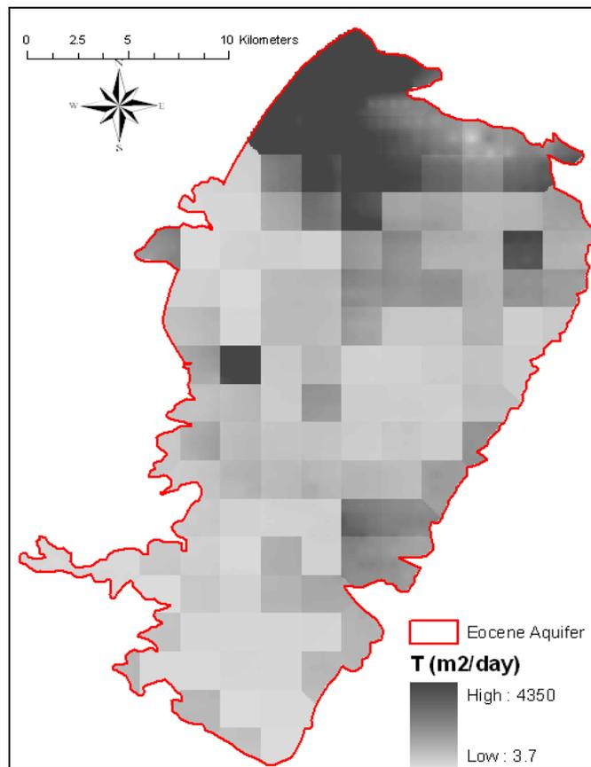
**Figure 7.12:** The Spatial Distribution of the Simulated Transmissivity Values
