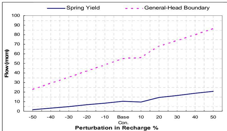
**Figure 7.26:** Sensitivity of Spring Yield and General-Head Boundary Outflow to Perturbations in the Groundwater Recharge
