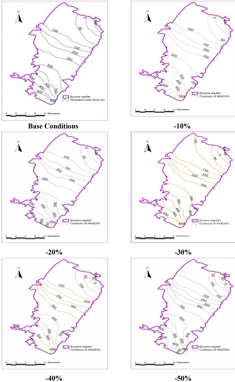
**Figure 7.16:** The Contours of Water Table Elevation for Different Decrease Percentages in the Hydraulic Conductivity Values
