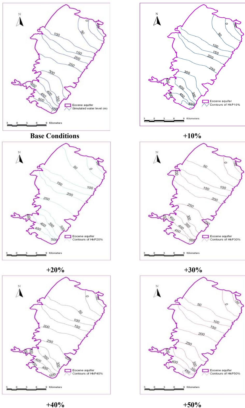
**Figure 7.15:** The Contours of Water Table Elevation for Different Increase Percentages in the Hydraulic Conductivity Values
