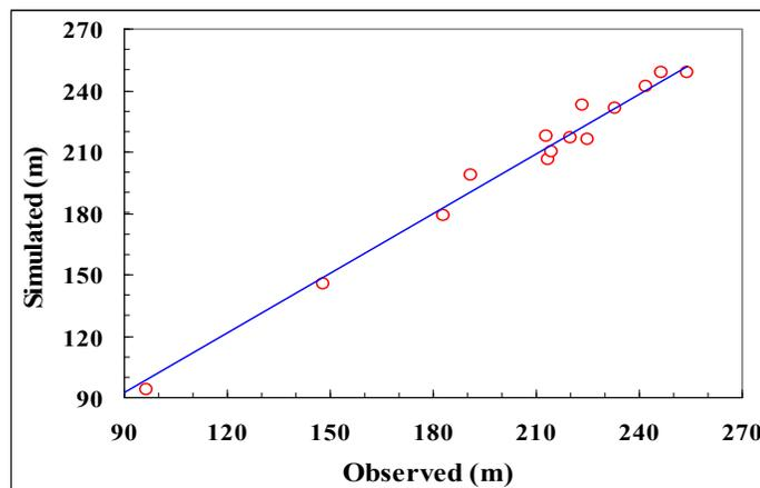
**Figure 7.14:** Simulated Versus Observed Water Table Elevations of the Eocene Model at the Calibration Locations
