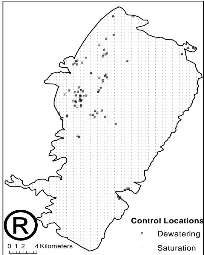
**Figure 8.3:** Control Point Locations for the Head Constraints for the Eocene Aquifer
