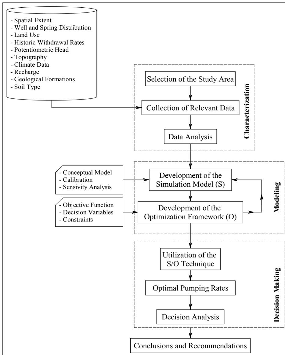
**Figure 6.1:** Flowchart of the Methodology for the Optimal Management of the Eocene Aquifer
