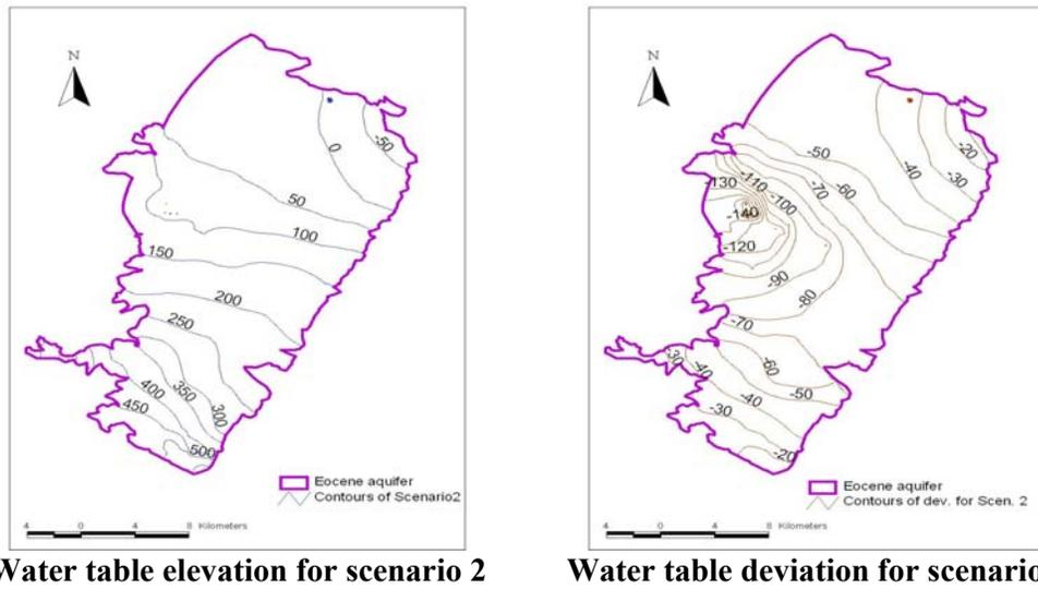
**Figure 8.7:** Contours of Water Table Elevation and its Deviation from the Simulated Model for Scenario 2
