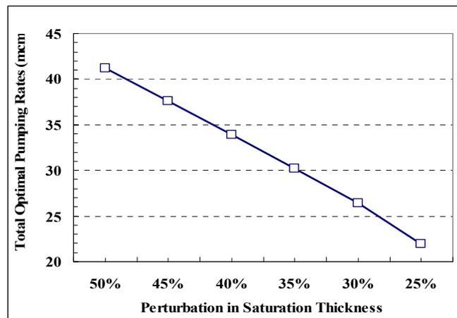
**Figure 8.13:** Optimal Pumping Rates for Different Reduction Percentages in the Minimum Saturation Thickness Requirement
