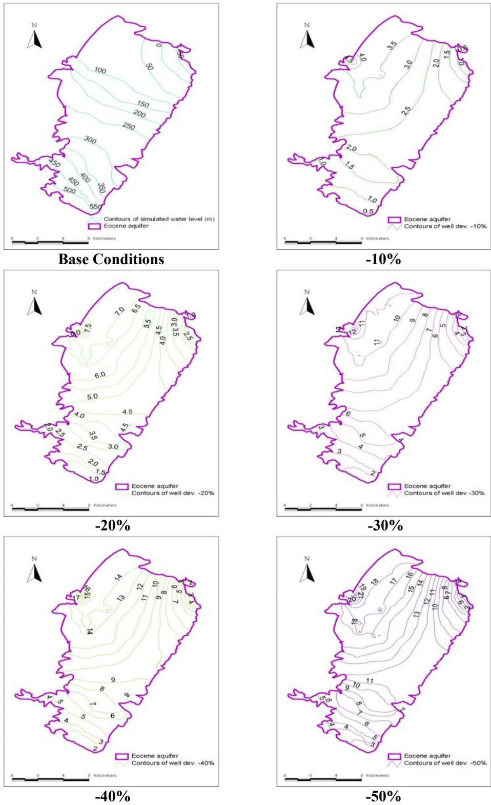
**Figure 7.30:** The Contours of Water Table Deviation for Different Decrease Percentages in Pumping Rates
