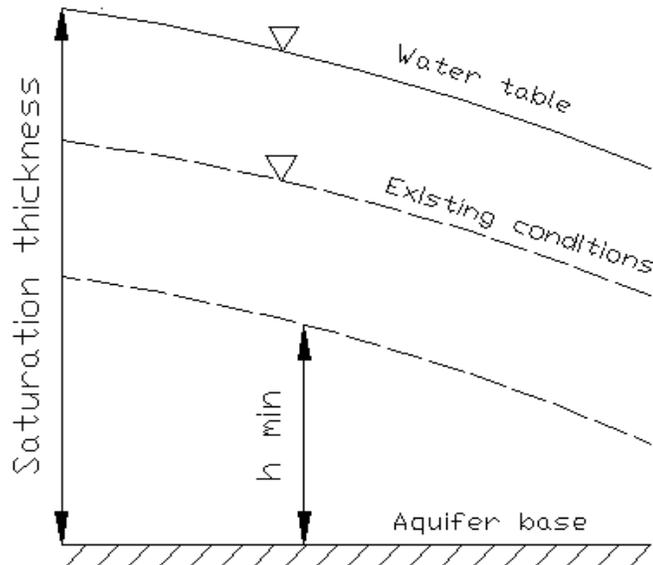
**Figure 8.2:** Head Constraint for the Eocene Aquifer Model
