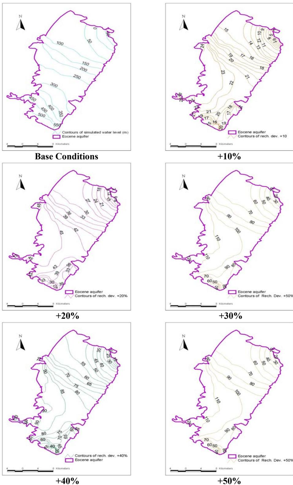
**Figure 7.23:** The Contours of Water Table Deviation for Different Increase Percentages in the Recharge Values
