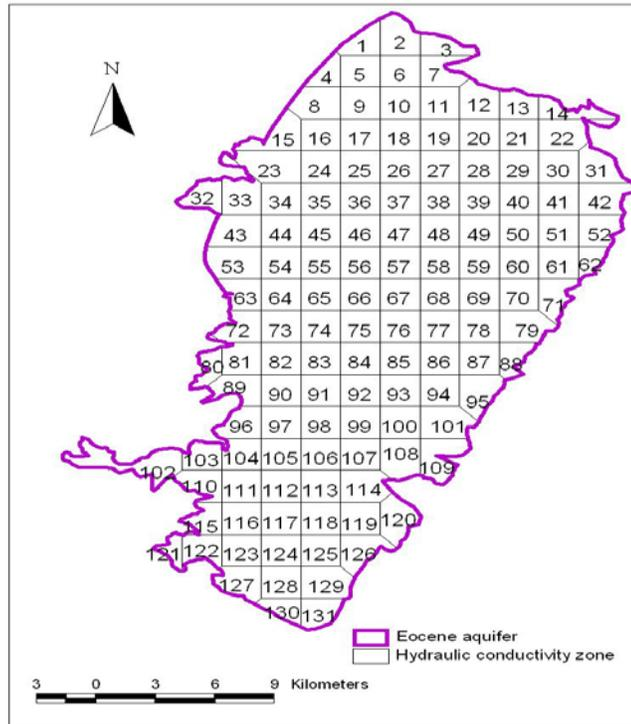
**Figure 7.10:** Hydraulic Conductivity Zones Utilized in Calibration. Numbers Indicate Zone ID
