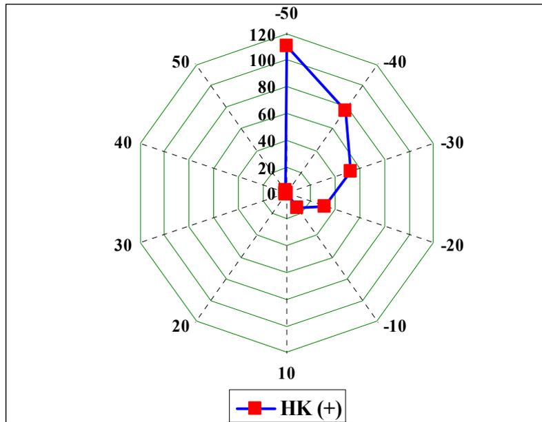
**Figure 7.34:** Positive Mean Deviation in Water Table Elevation for Different Perturbation Percentages in Hydraulic Conductivity
