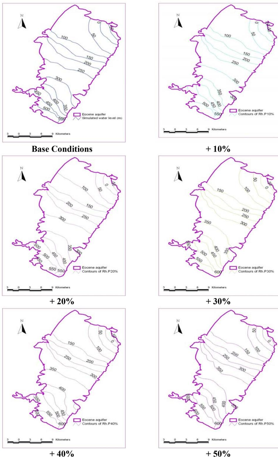
**Figure 7.21:** The Contours of Water Table Elevation for Different Increase Percentages in Groundwater Recharge
