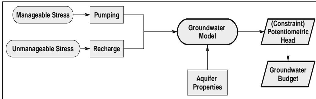
**Figure 4.1:** Simple Representation of a Groundwater Flow Model
