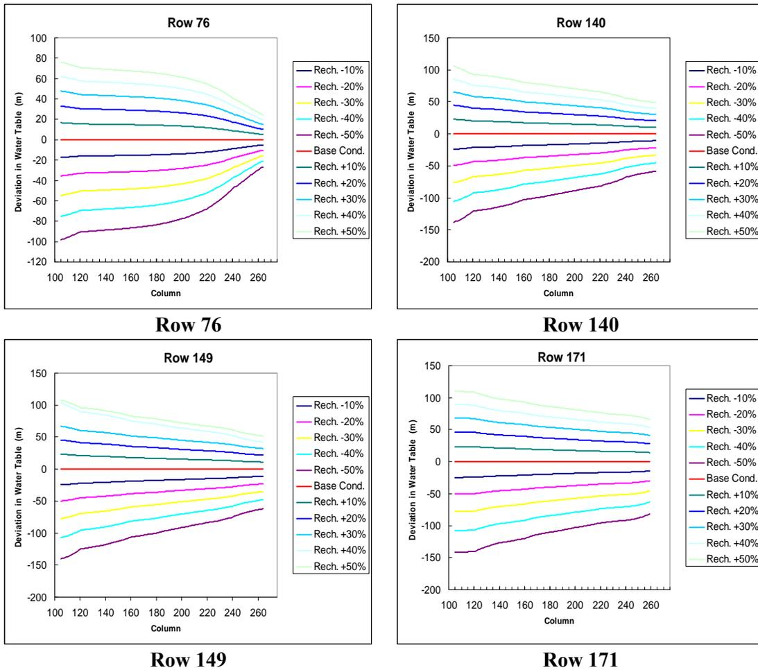
**Figure 7.25:** Deviation in Water Table Elevation for Specific Row and Column to Perturbations in the Groundwater Recharge
