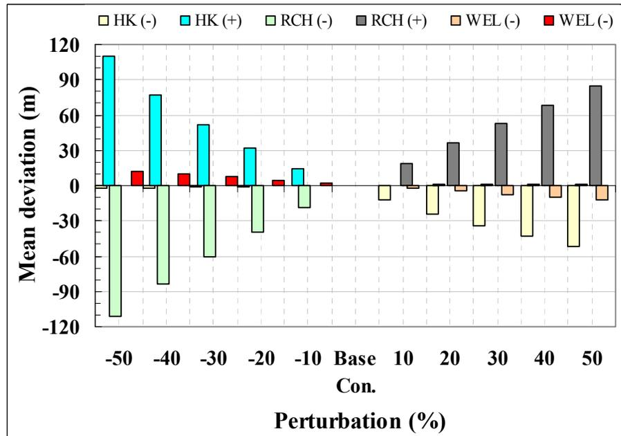
**Figure 7.33:** Mean Deviation in Water Table Elevation for Different Perturbation Percentages
