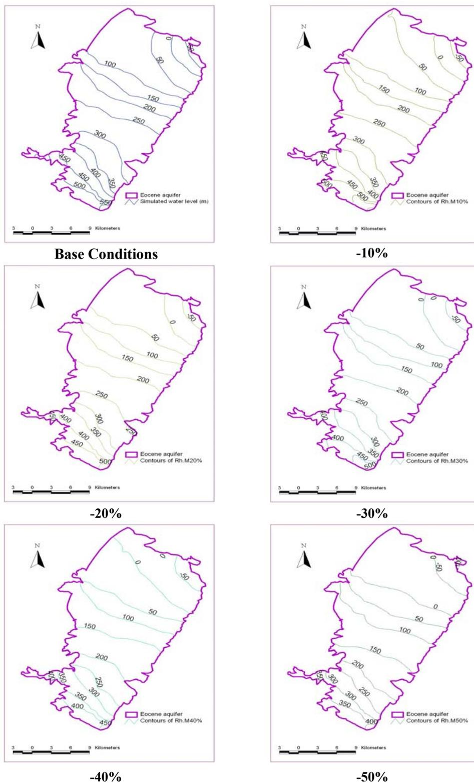
**Figure 7.22:** The Contours of Water Table Elevation for Different Decrease Percentages in Groundwater Recharge
