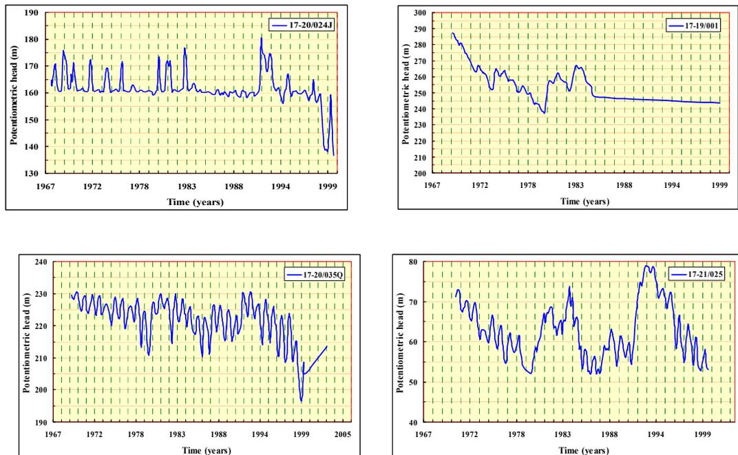
**Figure 7.8:** Time Series of Water Table Elevations for Selected Wells in the Eocene Aquifer
