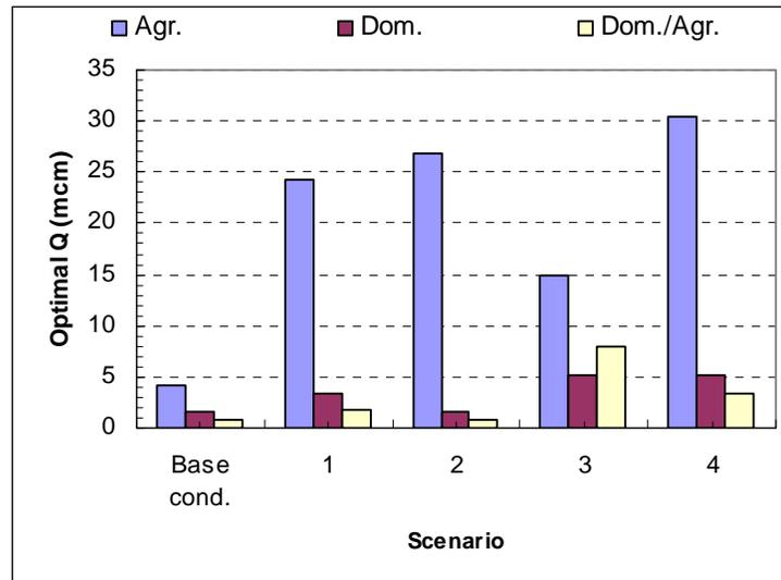
**Figure 8.10:** Optimal Pumping Rates for the Wells of the Eocene Aquifer as Classified According to Well Use under Different Management Scenarios
