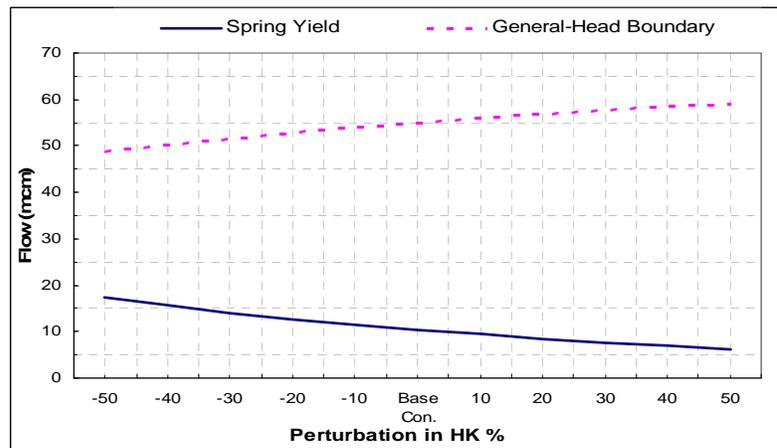
**Figure 7.20:** Sensitivity in Spring Yield and General-Head Boundary Outflow to Perturbations in the Hydraulic Conductivity
