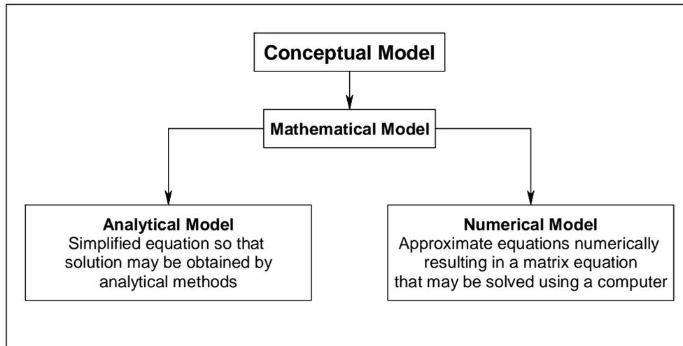
**Figure 4.3:** Logic Diagram for Developing a Mathematical Model
