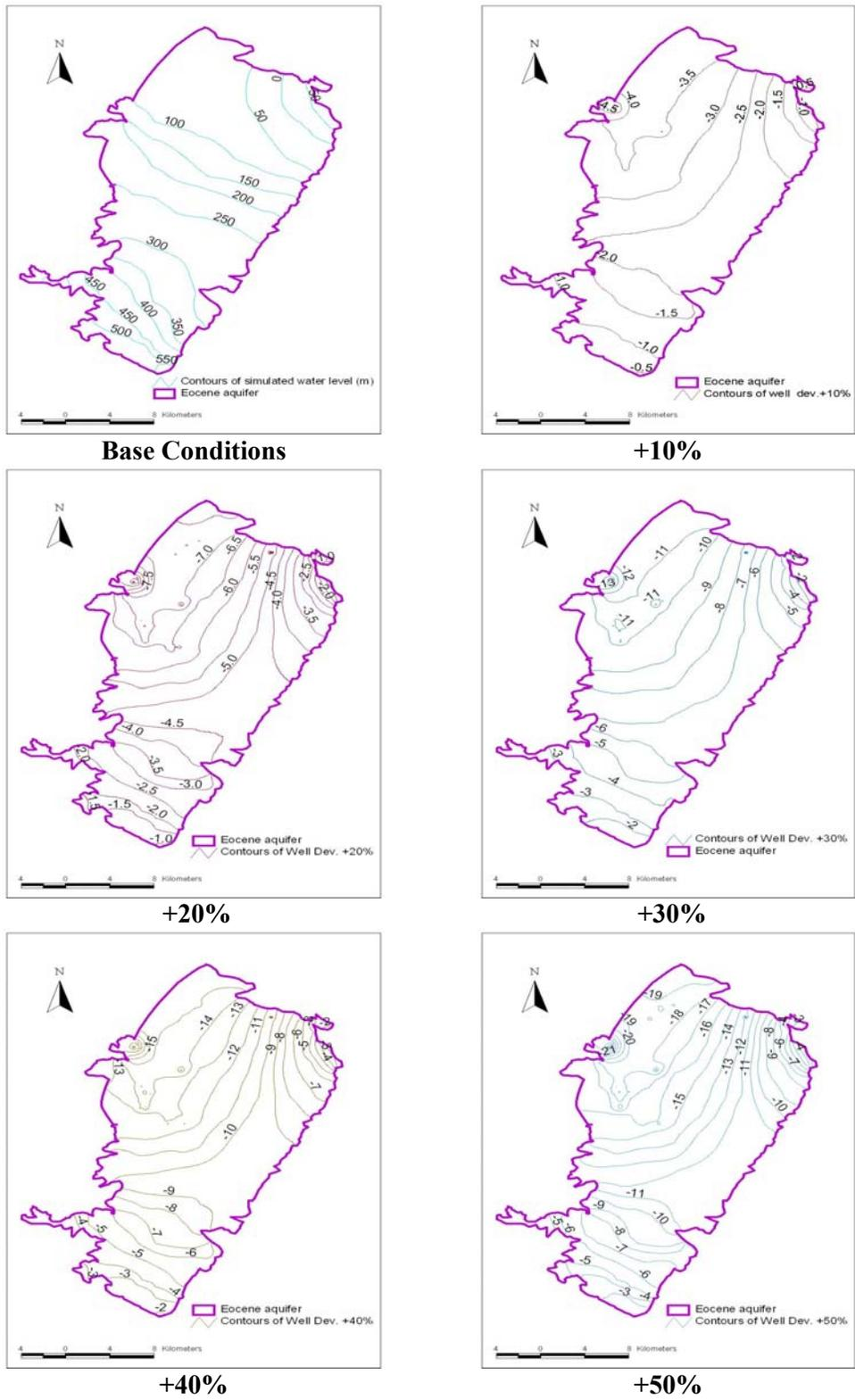
**Figure 7.29:** The Contours of Water Table Deviation for Different Increase Percentages in Pumping Rates
