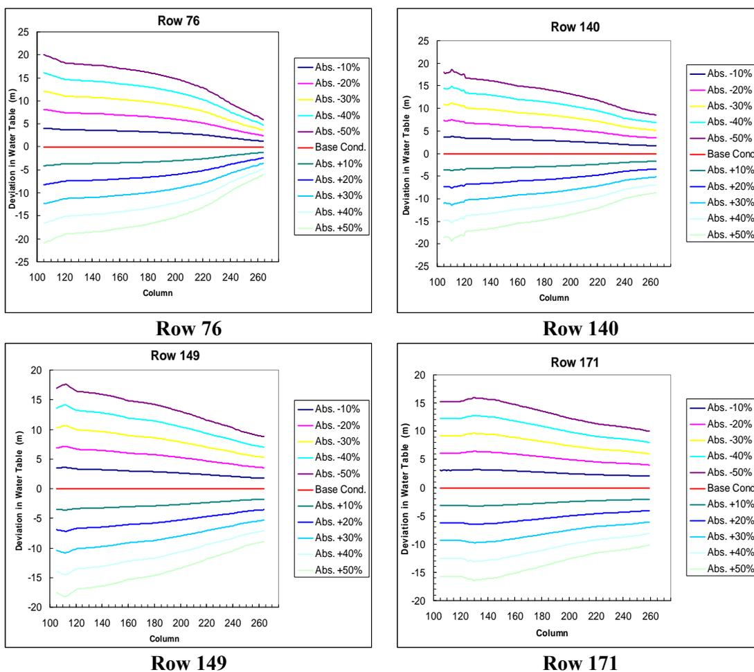
**Figure 7.31:** Deviation in Water Table Elevation for a Specific Row Due to Perturbations in Pumping Rates
