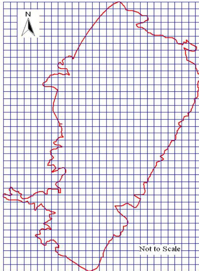
**Figure 7.1:** The Finite-Difference Grid of the Eocene Aquifer Model.
