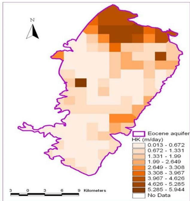
**Figure 7.11:** The Spatial Distribution of the Simulated Hydraulic Conductivity Values
