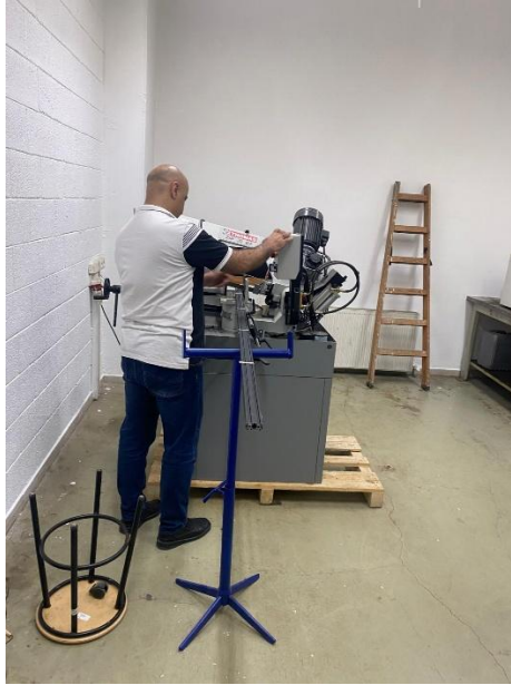
Figure 4: Cutting and preparing aluminum for the arena frame.
