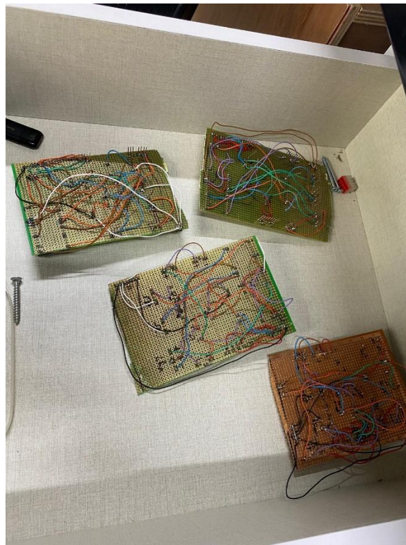
Figure 2: designed and soldered four custom circuits by hand to handle motor drivers, inputs, and power distribution.
