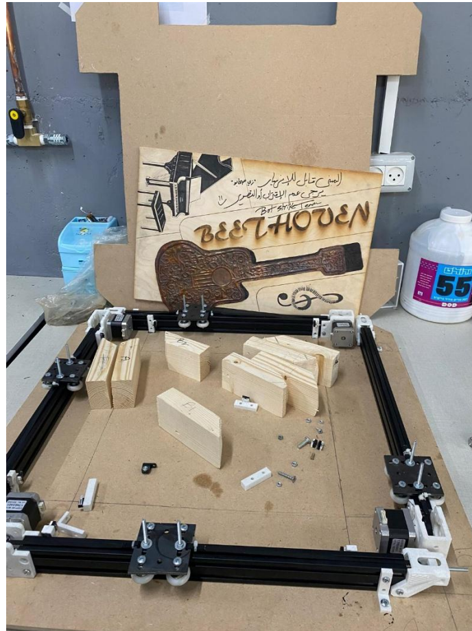
Figure 6: Mechanical assembly of the arena frame with mounted stepper motors.
