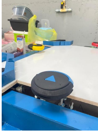
Figure 8: Close-up view of a player robot, showing the stepper motor mechanism.
