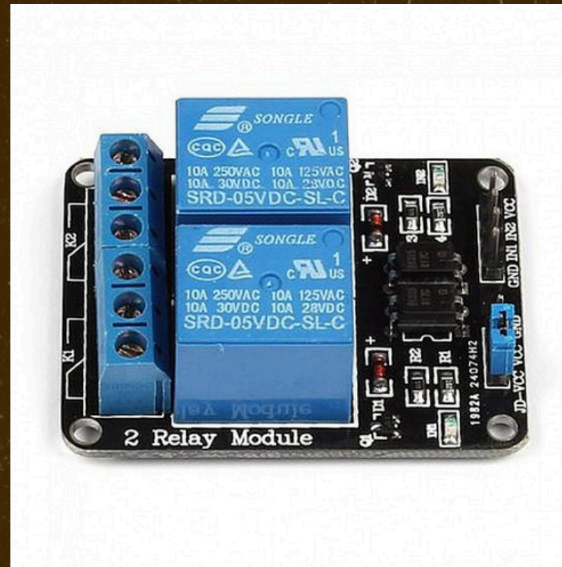
channel relay: for controlling heater and water pumps
