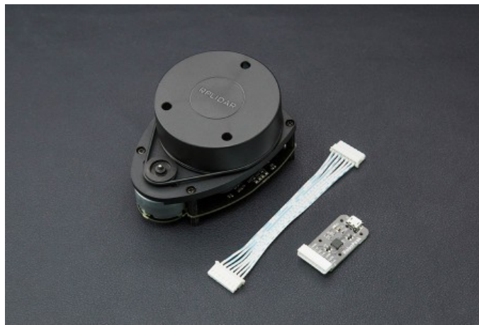
Figure 3.1: RPLIDAR A1 laser scanner used in this project.
