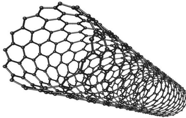
**Figure 1.2: A model of carbon nanotube molecule.**
