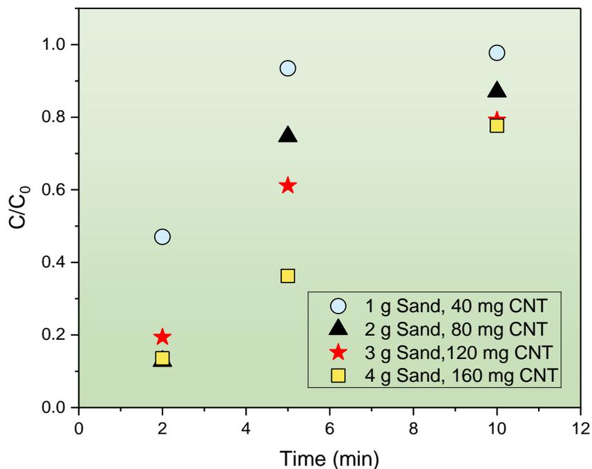
**Figure 3.6: Effect of bed-height on the adsorption on 25 ppm GPD adsorption, using constant ratio of silica to MWCNT at 25°C, and pH  $\approx$  7.**
