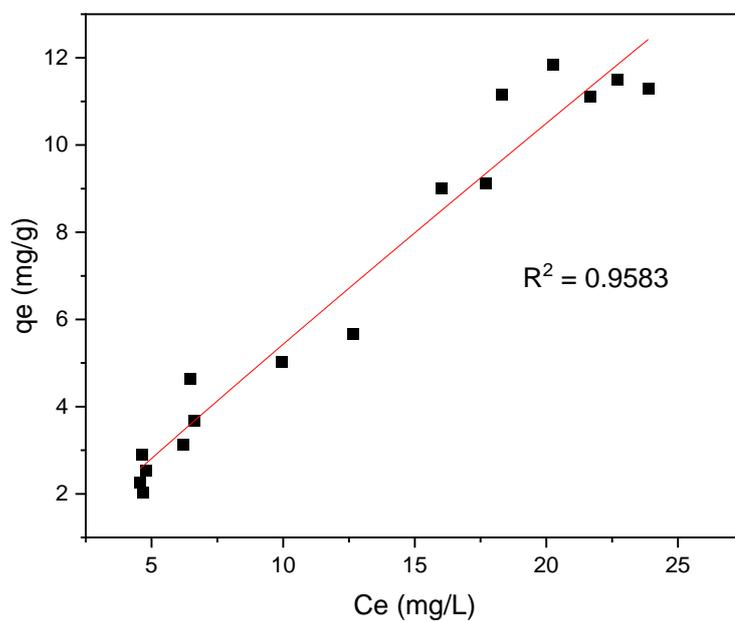
**Figure 3.4: Nonlinear fitting for the adsorption of 25 ppm GPD on MWCNT at room temperature based on the Freundlich model. Temp. = 25°C, pH  $\approx$  7.**
