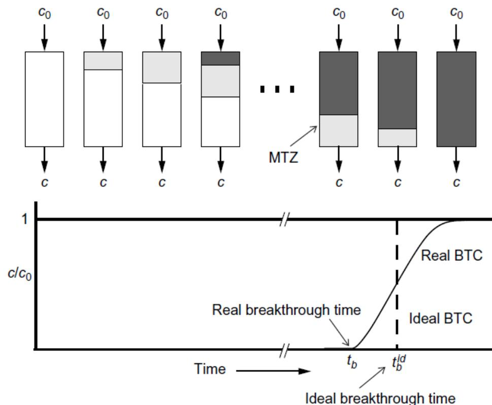
**Figure 2.2: Traveling of the mass transfer zone (MTZ) through the adsorber bed and development of the breakthrough curve (BTC). (Taken from Ref.51)**
