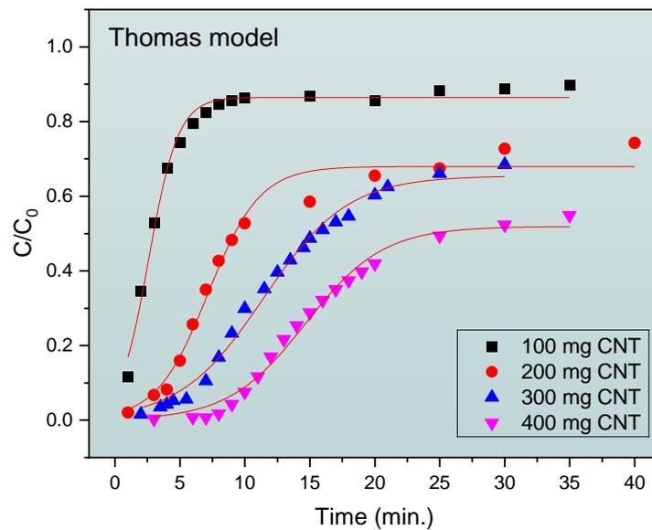
**Figure 3.10: Non-linear curve fitting according to the Thomas model for 25 ppm GPD adsorption at 25°C.  $\text{pH} \approx 7$ , bed-height= 3 cm.**
