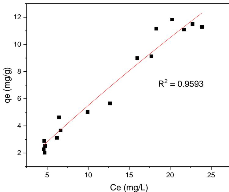
**Figure 3.3: Nonlinear fitting for the adsorption of 25 ppm GPD on MWCNT at room temperature based on the Langmuir model. Temp. = 25°C, pH  $\approx$  7.**
