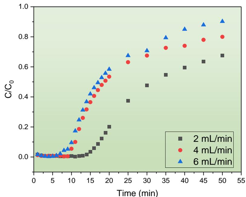
**Figure 3.7 : Effect of flow rate on the continuous adsorption of 25 ppm GPD at 25°C, and pH  $\approx$  7, MWCNT concentration = 400 mg, bed-height = 3 cm.**
