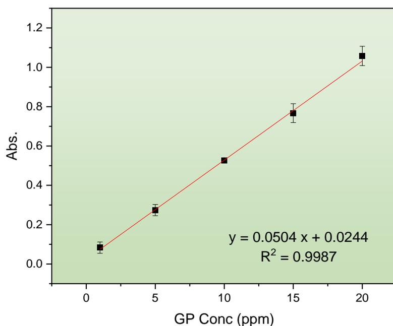
**Figure 3.2: Calibration curve for GPD standard solutions at 25°C, and pH  $\approx$  7.**
