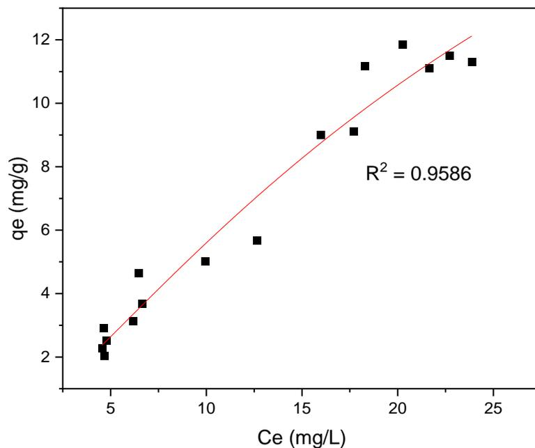
**Figure 3.5: Nonlinear fitting for the adsorption of 25 ppm GPD on MWCNT at room temperature based on the Sips model. Temp. = 25°C, pH ≈ 7.**
