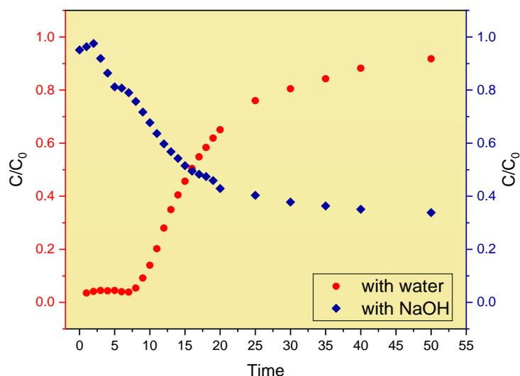
**Figure 3.11: Effect of regeneration, flush with 0.1M NaOH, distilled water, flush time= 15 min.**
