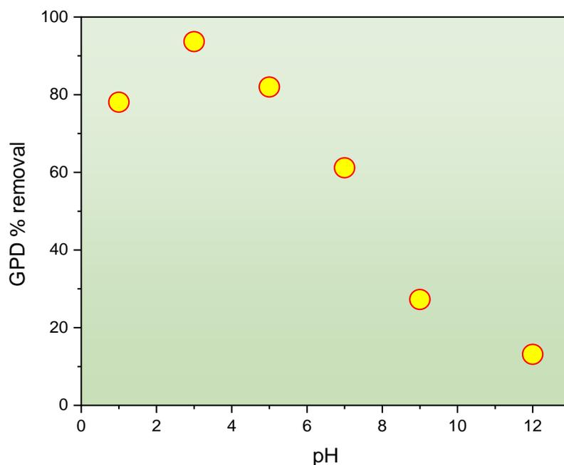
**Figure 3.8: Effect of solution pH on the batch adsorption of 25 ppm GPD at 25°C. MWCNT concentration = 50 mg, bed-height= 3 cm.**
