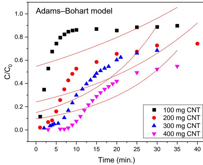
**Figure 3.9: Non-linear curve fitting according to the Adams–Bohart model for 25 ppm GPD adsorption at 25°C.  $\text{pH} \approx 7$ , bed-height= 3 cm.**
