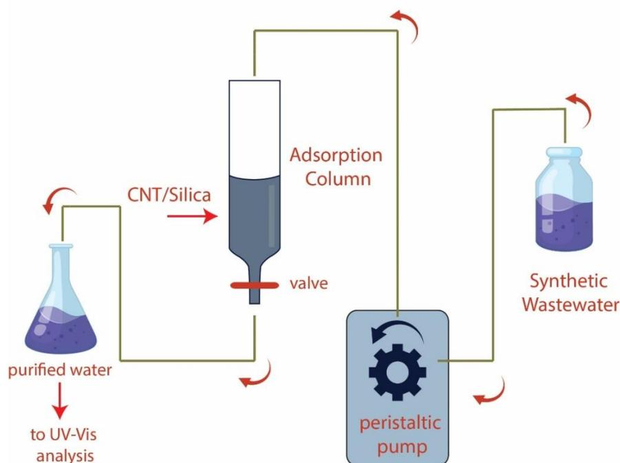
**Figure 2.1: Experimental setup for the continuous adsorption**
