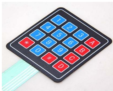
Figure 24 4 x 4 Matrix Keypad
