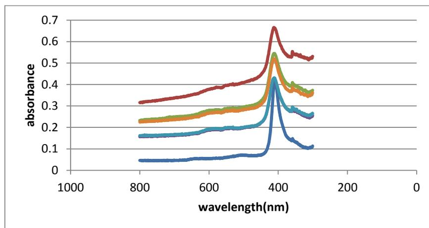
**Figure (3. 18):** Absorbance vs. wavelength(nm) of Mb. (Different conc. of  $\text{Cu}^{2+}$  (0.0002, 0.0004, 0.0005, 0.0006, 0.0008, and 0.001M) with 50 ppm myoglobin in presence of membrane.
