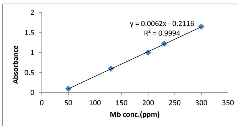
**Figure (3. 21):** calibration curve for Mb- Cu<sup>2+</sup>-complex at pH 7.3, 400 nm.
