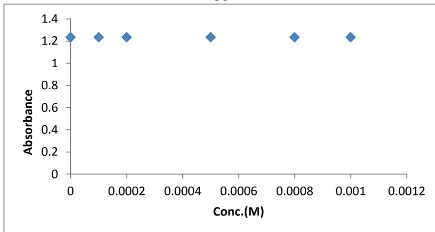
**Figure (3. 13):** Sensor response to Na<sup>+</sup> at pH=7.3, at RT, and 400nm.
