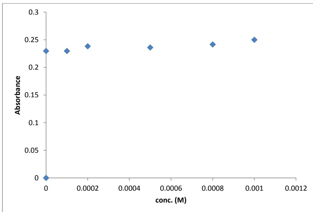
**Figure (3. 8):** Turbidity absorbance of sensing element vs concentration of  $\text{Co}^{2+}$  in distilled water at 400 nm, 25 °C, pH~7.3.
