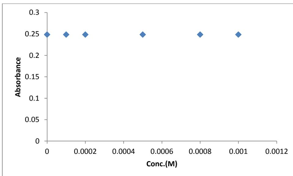
**Figure (3. 10):** Turbidity absorbance of sensing element vs concentration of ( $\text{Hg}^{2+}$ ) in distilled water at 400 nm, 25 °C, pH~7.3.
