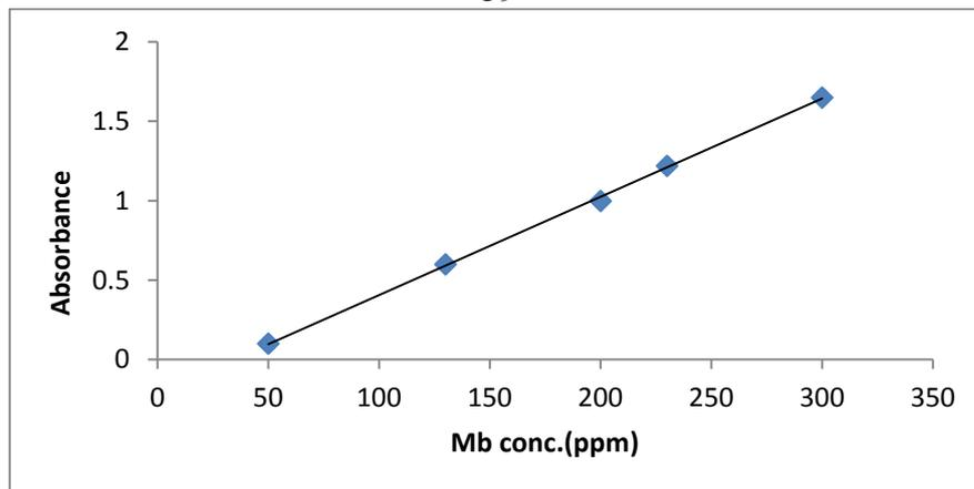
**Figure (3. 20):** Response of sensing membrane to different conc. of myoglobin( 50, 130, 200, 230, 300ppm), (0.001M Cu<sup>2+</sup>) .
