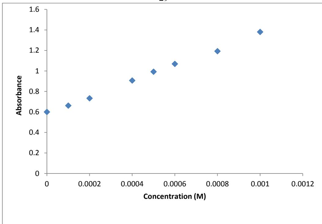
**Figure (3. 7):** Turbidity absorbance of sensing element vs concentration of  $\text{Cu}^{2+}$  in distilled water at 400 nm, 25 °C, pH~7.3.
