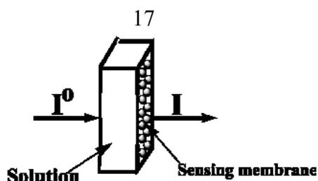
Figure (2. 1): optical sensing system
