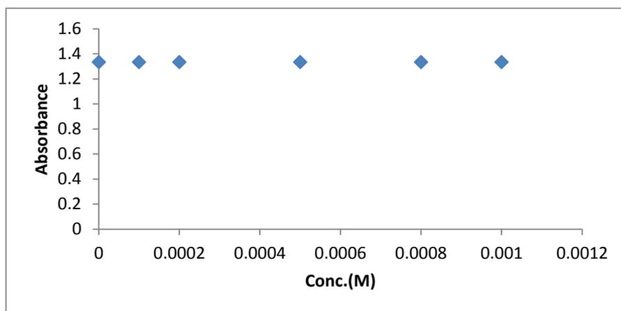
**Figure (3. 14):** Sensor response to K<sup>+</sup> at pH=7.3, at RT, and 400nm.
