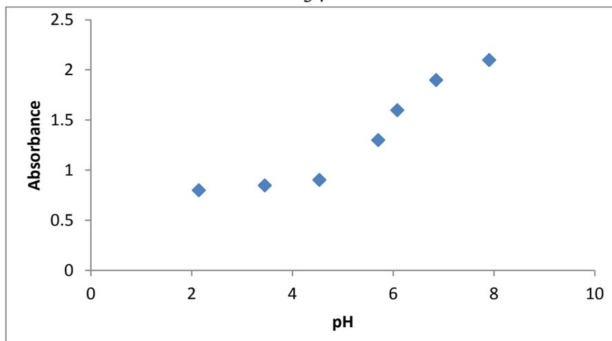
**Figure (3. 12):** Turbidity absorbance of the sensing element for (0.001M) Cu<sup>2+</sup> at different pHs.
