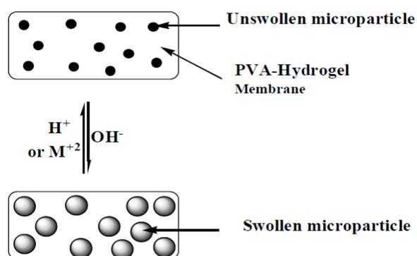
**Figure (3. 2):** Schematic diagram of sensing response to pH and metal ions
