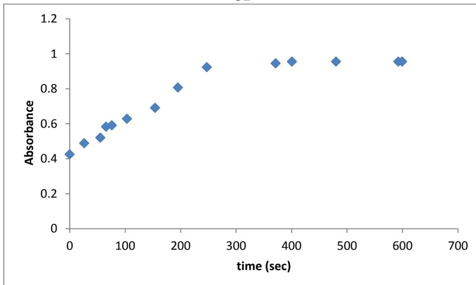
**Figure (3. 11):** The response time of the sensing membrane of  $\text{Cu}^{2+}$  in distilled water (pH~7.3).
