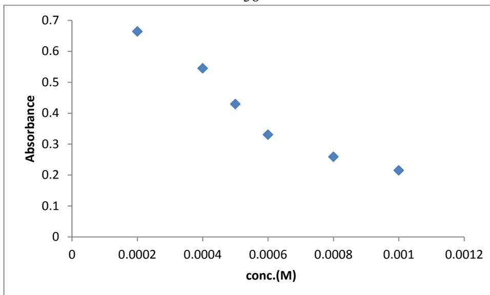
**Figure (3. 19):** Turbidity absorbance of the sensing element for Mb (50ppm) of different concentrations of  $\text{Cu}^{2+}$  (0.0002, 0.0004, 0.0005, 0.0006, 0.0008, and 0.001ppm) in distilled water (pH=7.3),  $\lambda=400$ , and at room temperature.
