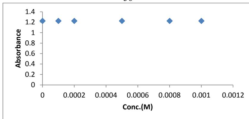
**Figure (3.16):** Sensor response to Ca<sup>2+</sup> at pH=7.3, at RT, and 400nm.
