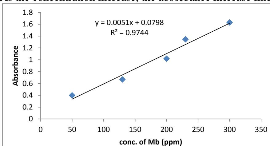
**Figure (3.17):** Sensor response of different concentrations of myoglobin (50, 130, 200, 230, and 300ppm) at  $\lambda=400$ , in distilled water (pH= 7.3) without membrane.
