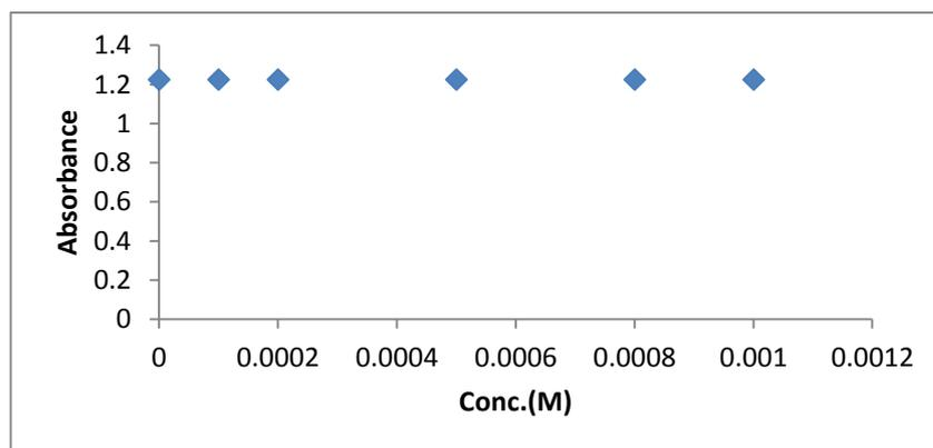
**Figure (3. 15):** Sensor response to Mg<sup>2+</sup> at pH=7.3, at RT, and 400nm.
