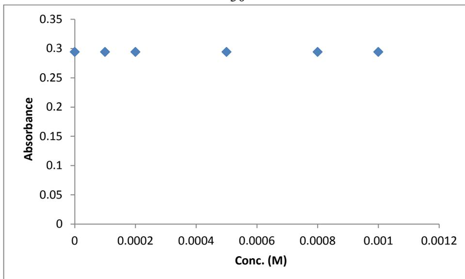
**Figure (3. 9):** Turbidity absorbance of sensing element vs concentration of ( $\text{Ni}^{2+}$ ) in distilled water at 400 nm, 25 °C, pH~7.3.
