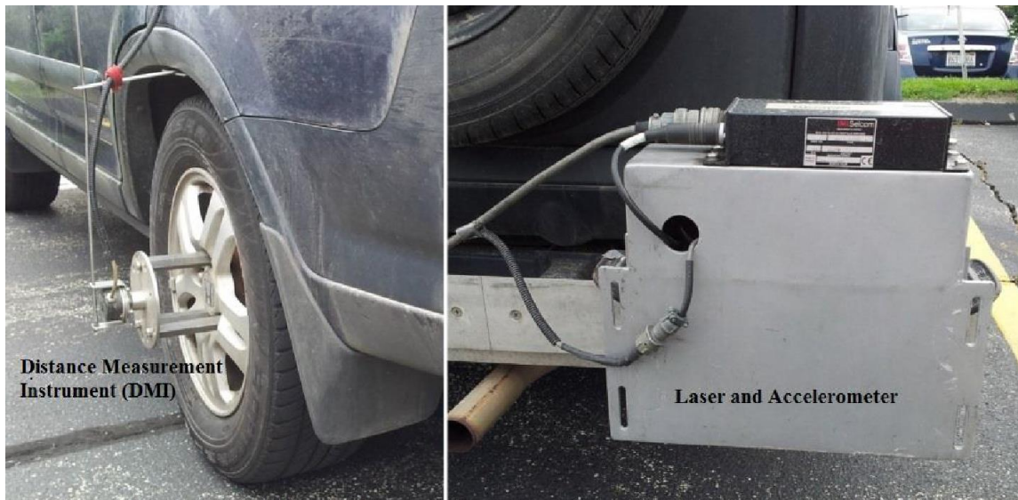
Figure 2.1: Automated Pavement Profiler and Equipment on a Typical Data Collection Van
