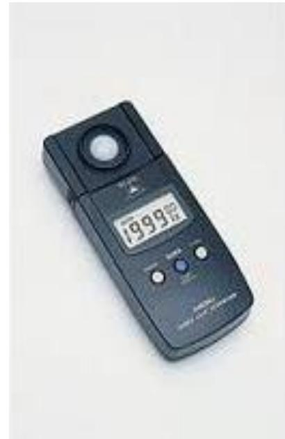
Lux meter depend on photo cell to hold the light then it converts it into an electrical current, and by measuring this current allows the device to calculate the lux value of the
