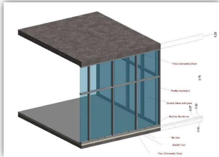
Figure 123 : The installation detail in Revit
