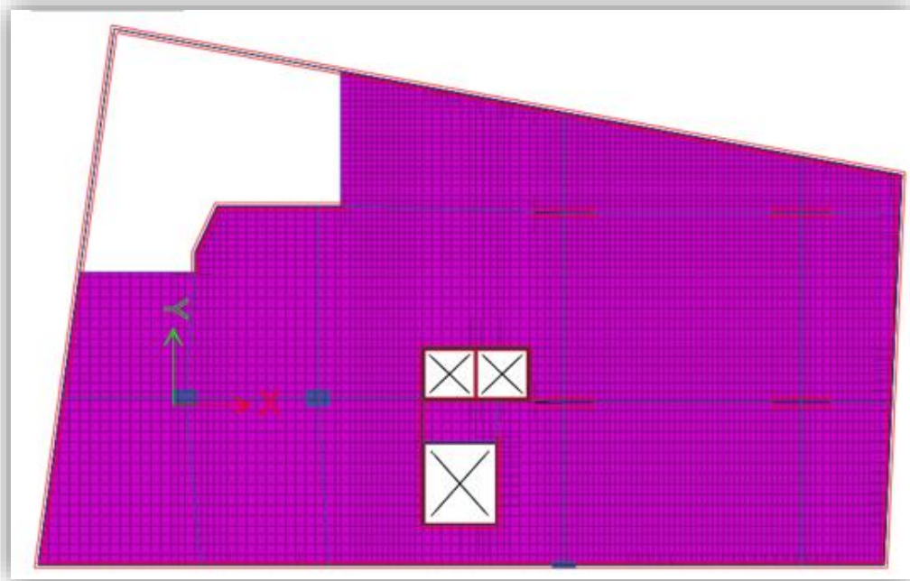
Figure 210: The bottom reinforcement in Basement 3 floor in x direction.
