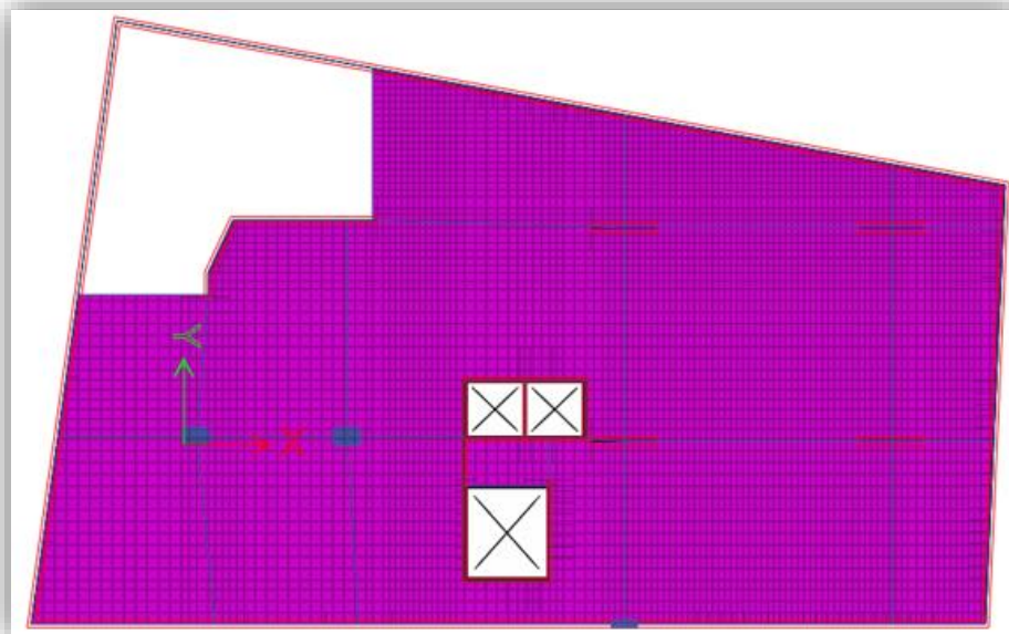
Figure 209: The top reinforcement in Basement 3 floor in x direction.
