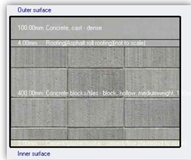
Figure 107:Layers and thickness for the roof before insulation
