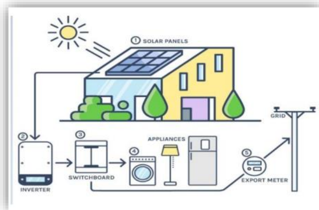
Figure 142: Solar PV system
