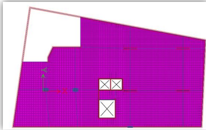
Figure 212: The bottom reinforcement in Basement 3 floor in y direction.
