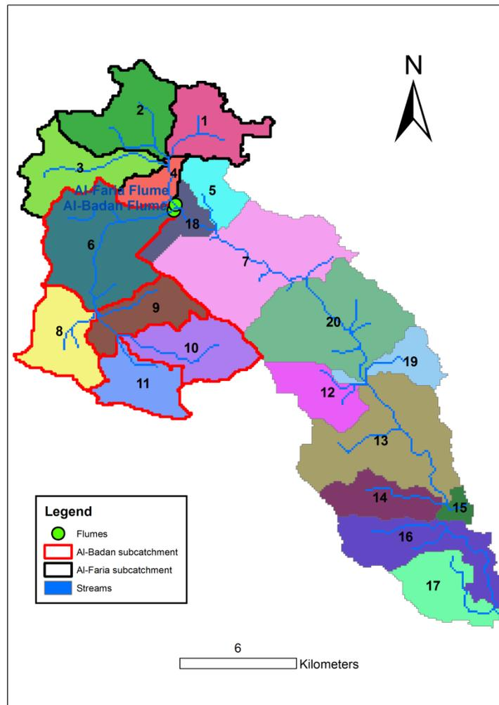
**Figure (5. 4):** Sub-catchments for HEC-HMS model
