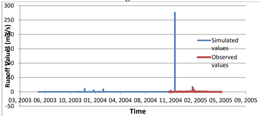
**Figure (5. 19):** Simulated and observed hydrographs for Badan sub-catchment
