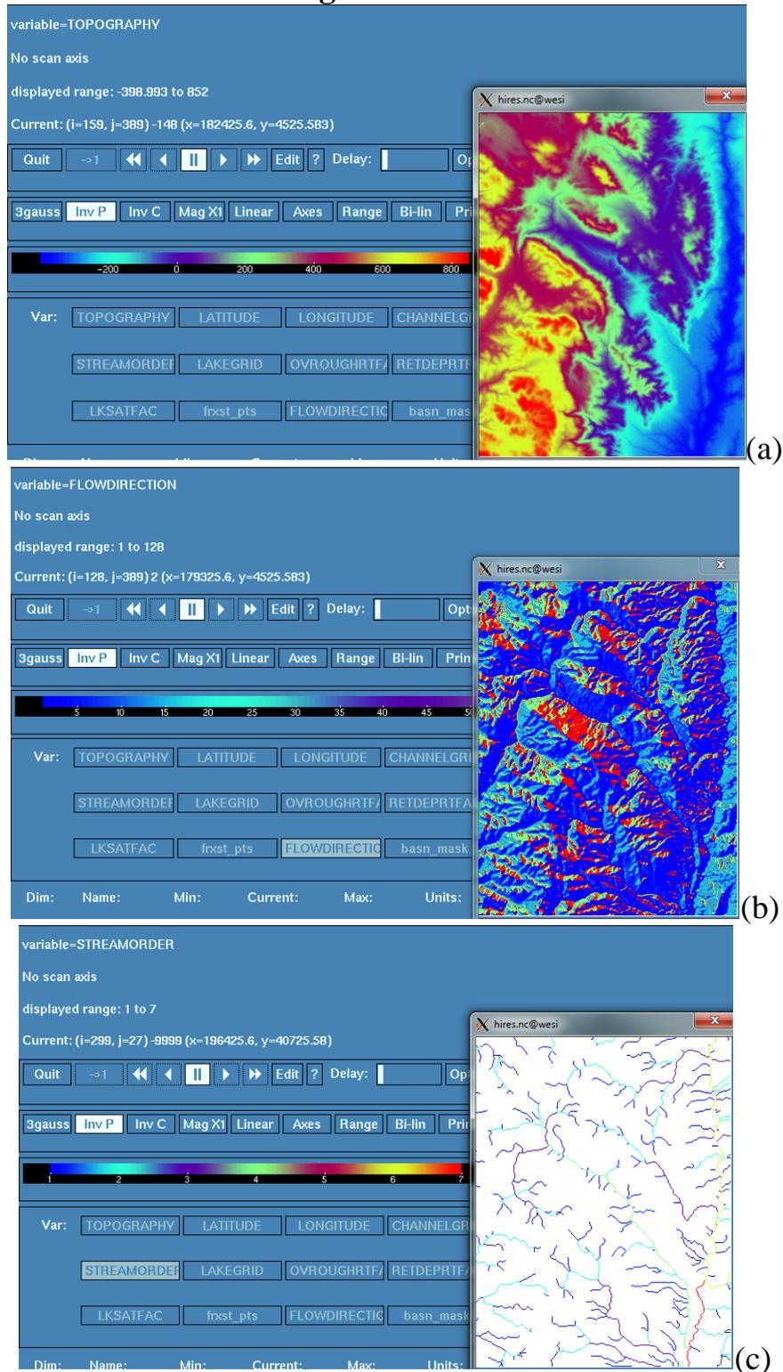
**Figure (5. 13):** Terrain routing data including: (a) Topography, (b) Flow direction, and (c) Stream order
