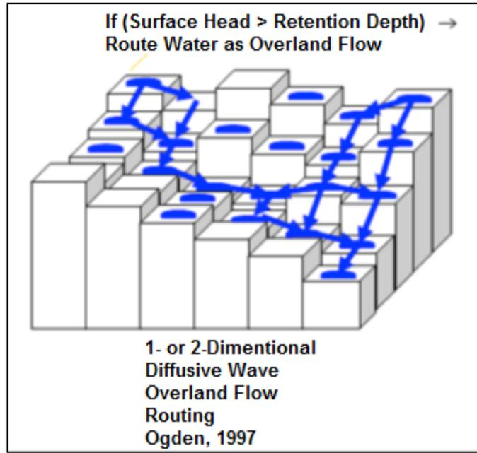
**Figure (5. 8):** Overland flow routing module in Noah LSM
