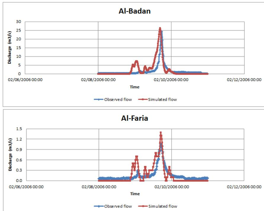
**Figure (5. 7):** Observed and Simulated flows for 8-10, February, 2006
