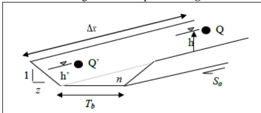
**Figure (5. 11):** Schematic of channel routing terms
