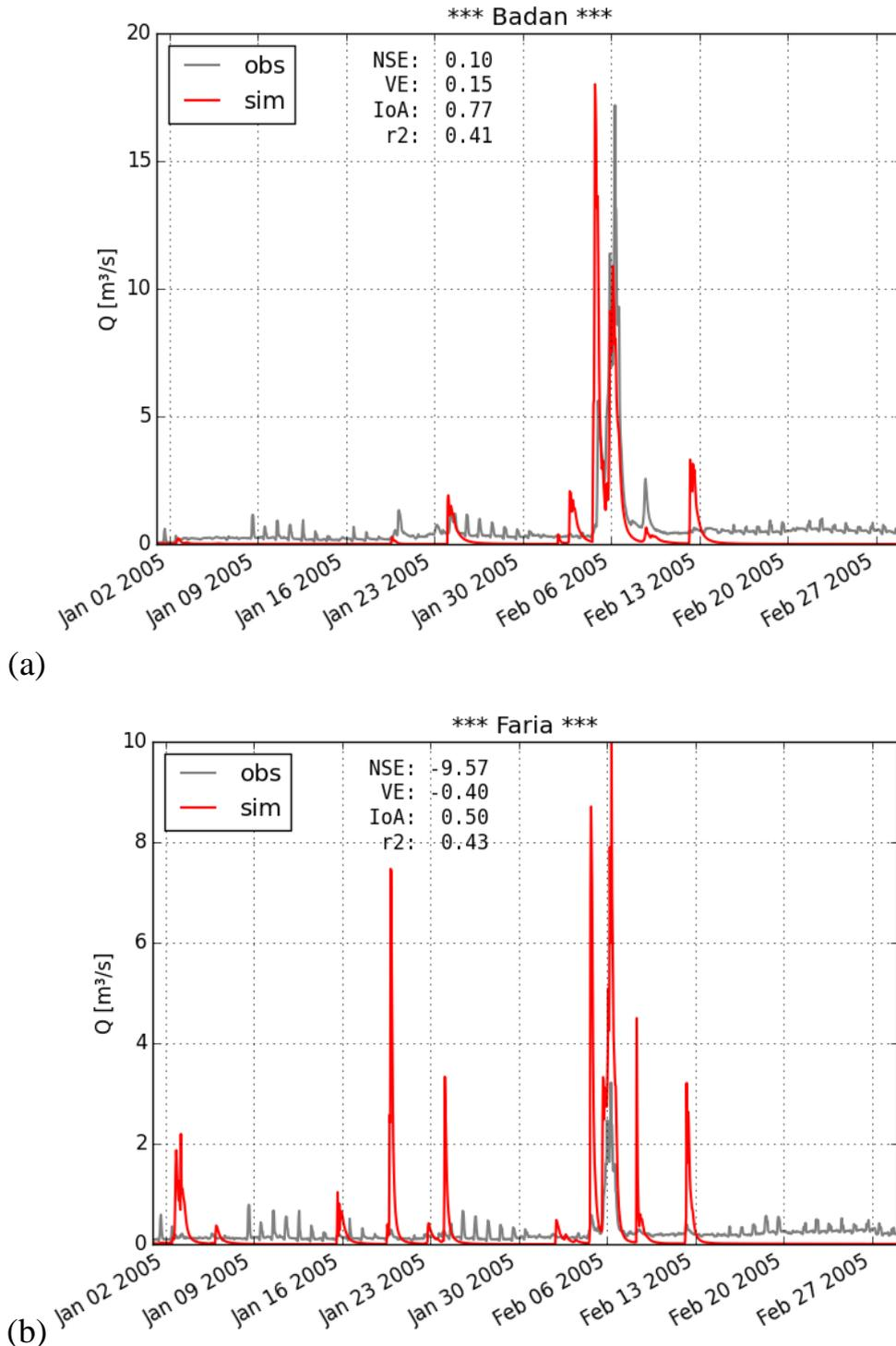
**Figure (5. 16):** Simulation hydrographs for the period of (Jan and Feb, 2005) for the sub-catchments of (a): Al-Badan, and (b) Al-Faria
