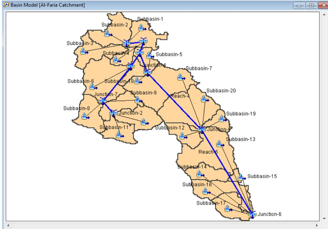
**Figure (5. 5):** Faria catchment hydrologic model using HEC-HMS v.4
