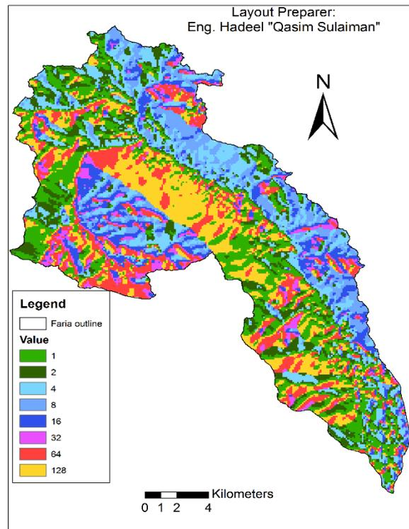
**Figure (5. 2):** Eight direction flow model **Figure (5. 3):** Flow Direction map of Faria catchment
