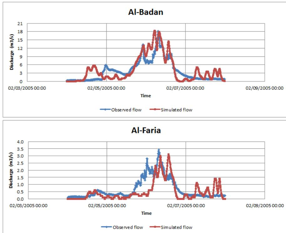
**Figure (5. 6):** Observed and Simulated flows for 4-8, February, 2005
