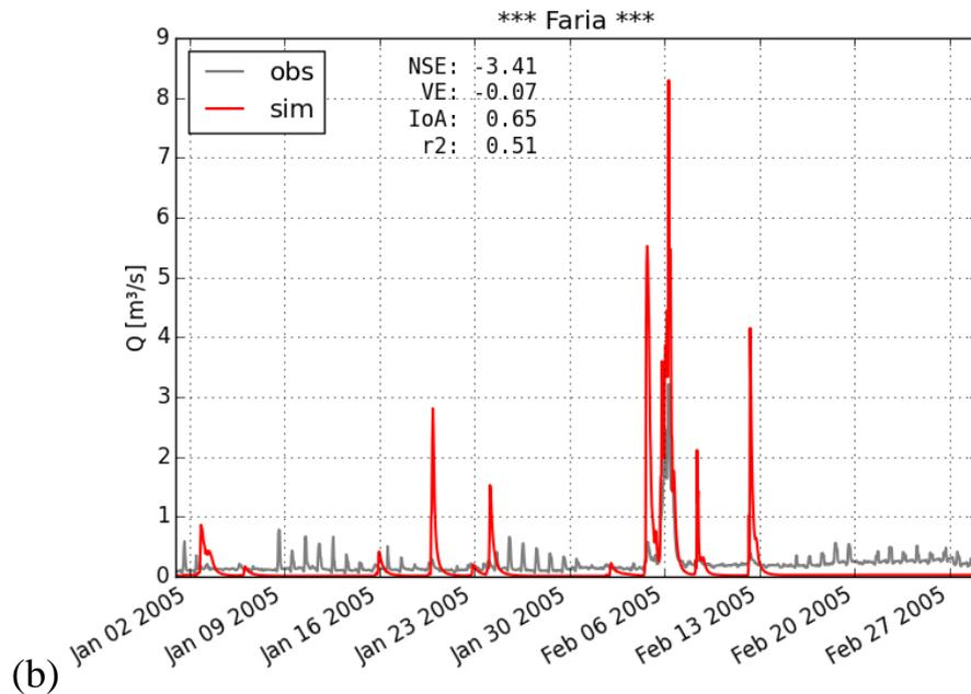
**Figure (5. 18):** Simulation hydrographs for the period of (Jan and Feb, 2005) after calibration for the sub-catchments of (a): Al-Badan, and (b) Al-Faria
