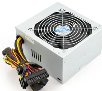
Figure 12: ATX power supply unit used as the primary system power source.
