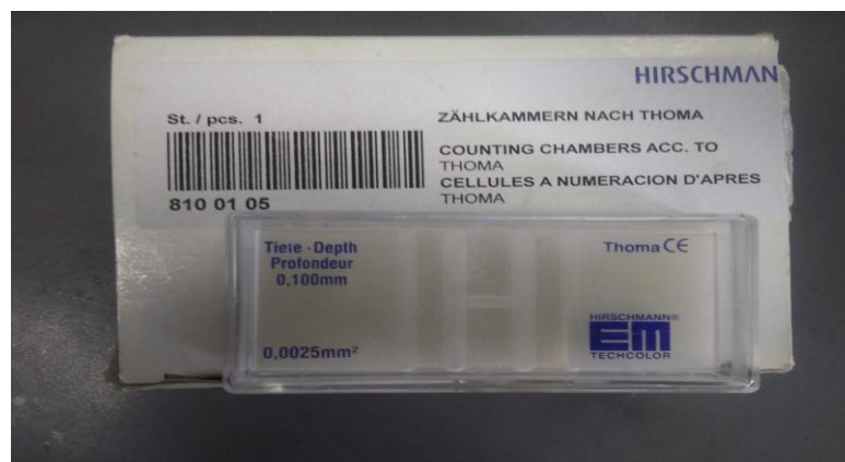
Figure 9. Micrometer slide used to calculate CFU/ML of free cell
