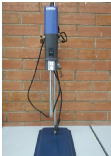
Figure 10. plate heater was used as a way Figure 11: Ultraturrax homogenizer for mechanical stirring by using magnetite
