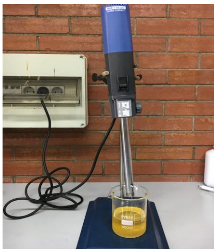
Figure 18. Ultraturrax and the mix of oil, alginate and yeast cells.
