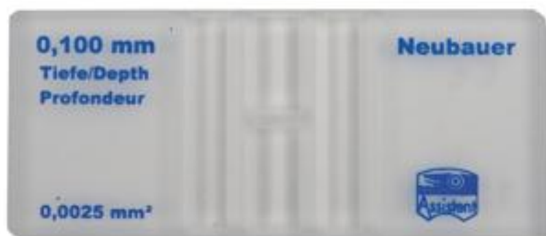
Figure 22. Micrometer slide used for numbering and size calculation of microcapsules.
