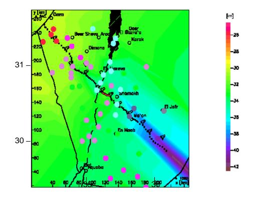
**Figure 9.** Moho depth map beneath the 3-dimensional gravity modelling area of the Dead Sea Transform (contour interval 0.5 km, scale 1:30000). Also shown is the moho depth (circles) from the receiver function data (19).
