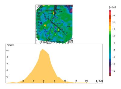
**Fig** *Iistogram of gravity differences between measured and computed Bouguer anomalies (correlation coefficient 0.98). Also shown is the misfit between the measured and computed Bouguer anomaly map of the study area (contour interval 1 mGal).*
