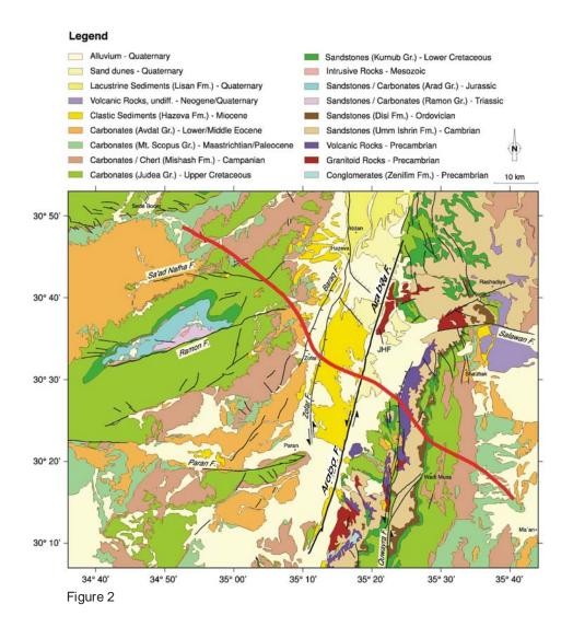
**Figure 2.** Geological Map of the modelling planes, the red line represents the near-vertical seismic reflection profile (35).
