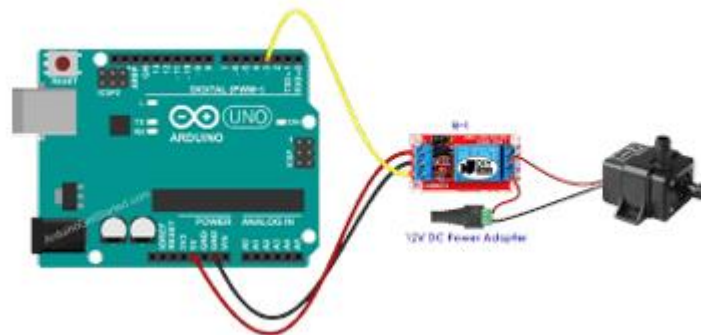
Figure 4.3: Water pump connection
