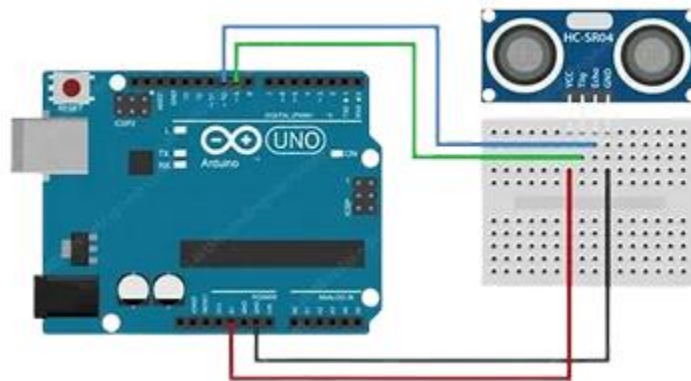
Figure 4.7: Ultrasonic Sensor Connections.
