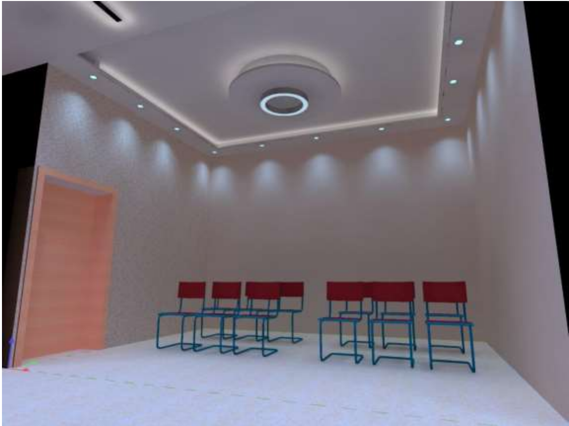
Figure 201 - Waiting Area 2 Lighting Distribution (DiaLUX)
