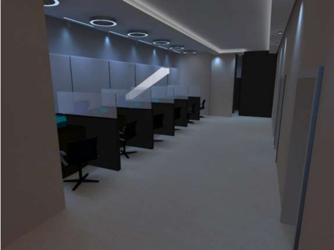
Figure 195 - Tellers Lighting Distribution (DiaLUX)
