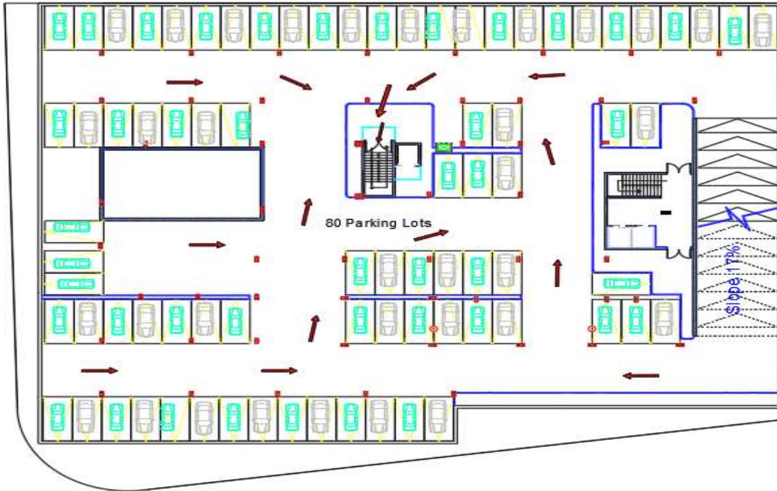
Figure 46 - Escape routes in Basement Level 2
