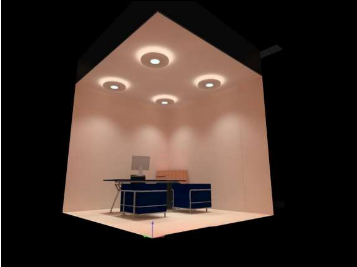
Figure 200 - Office Lighting Distribution (DiaLUX)
