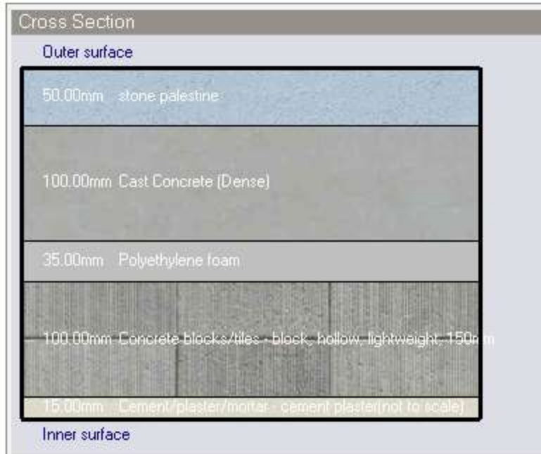
Figure 81 - external wall layers (after Modification)
