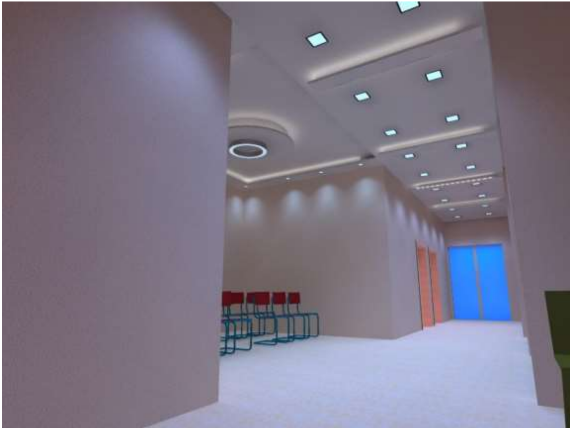
Figure 202 - Corridor Lighting Distribution (DiaLUX)
