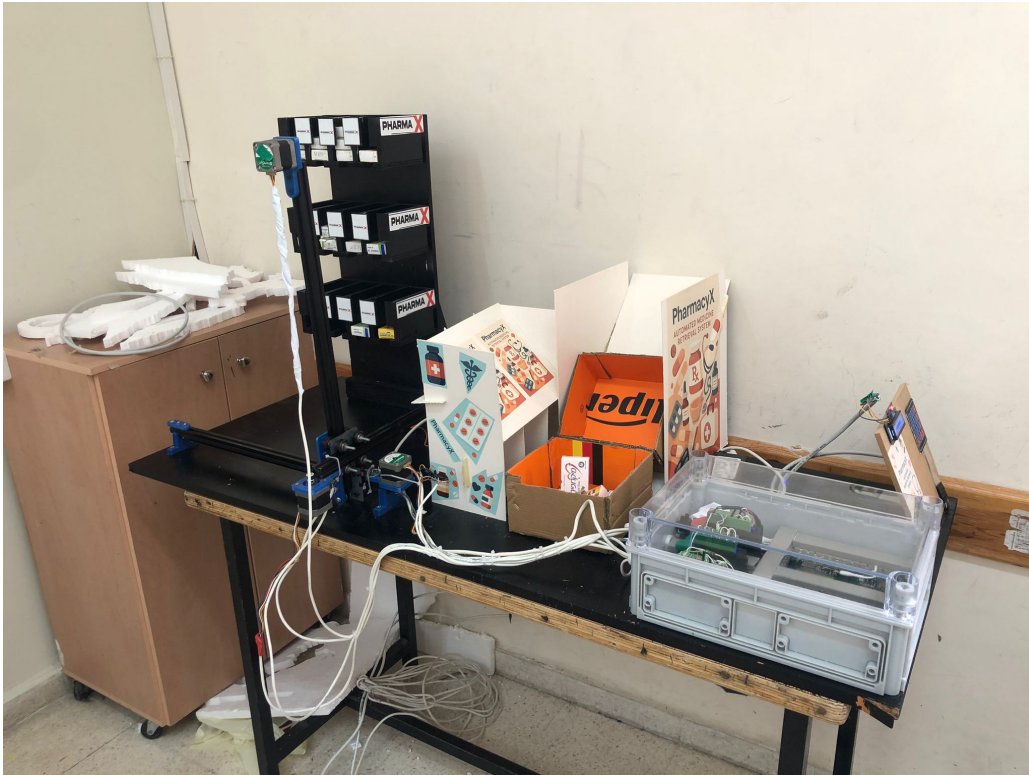
Figure 1: PharmaX: three-axis gantry, 3 \times 4 shelves, Z-platform with pusher, and gravity ramp to the user bin.
