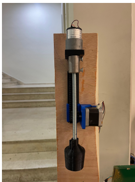
Figure 3.14: Capping process Stage 2: Sealing the Cap
