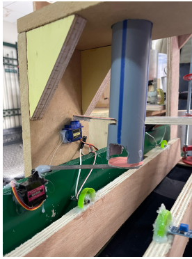
Figure 3.12: Capping Process Stage 1: Dropping the Cap
