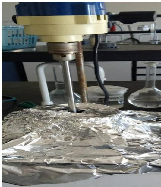
**Figure 2.1:** Apparatus for oxidation of cellulose
