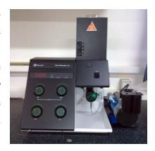
Before use, the device requires calibration with a series of standard solutions of the ion to be tested. Flame photometry is crude but cheap compared to flame emission spectroscopy, where the emitted light is analysed with a monochromator. Its status is similar to that of the colorimeter (which uses filters) compared to the spectrophotometer (which uses a monochromator). It also has the range of metals that could be analysed and the limit of detection is also considered.
