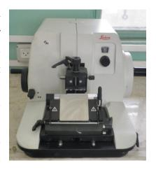
sections of animal or plant tissues for light microscopy histology. Glass knives are used to slice sections for light microscopy and to slice very thin sections for electron microscopy. Industrial grade diamond knives are used to slice hard materials such as bone, teeth and plant matter for both light microscopy and for electron microscopy. Gem quality diamond knives are used for slicing thin sections for electron microscopy.
