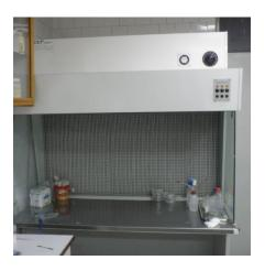
many different types of cabinets with a variety of airflow patterns and acceptable uses. NSF49 is the commonly accepted regulatory standard for these cabinets. Laminar flow cabinets may have a UV-C germicidal lamp to sterilize the shell and contents when not in use.
