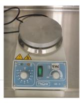
quickly, agitating or mixing the liquid. A magnetic stirrer often includes a provision for heating the liquid.
