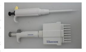
piece glass pipettes to more complex adjustable or electronic pipettes. Many pipettes types work by creating a partial vacuum above the liquid-holding chamber and selectively releasing this vacuum to draw up and dispense. Pipettes that dispense between 1 and 1000 µl are termed micropipettes, while *macropipettes* dispense a greater volume of liquid.
