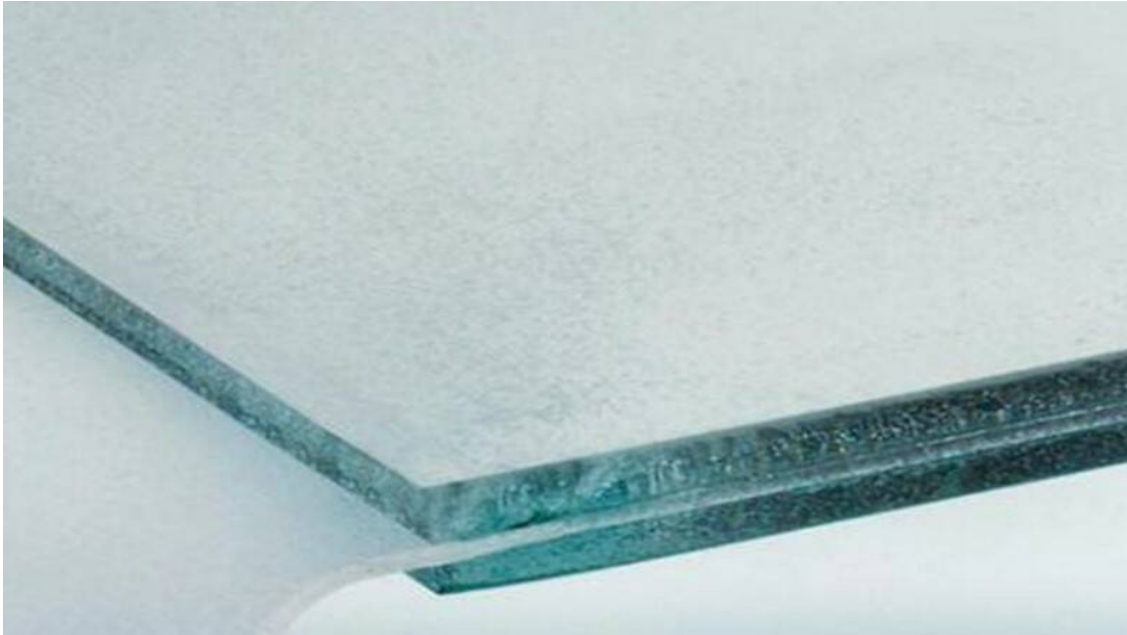
Figure 2-3: Thermochromic glass in production with a PVB layer sandwiched between two glass layers.
