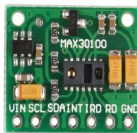
Figure2 Max30100 spo2 and heart rate sensor
