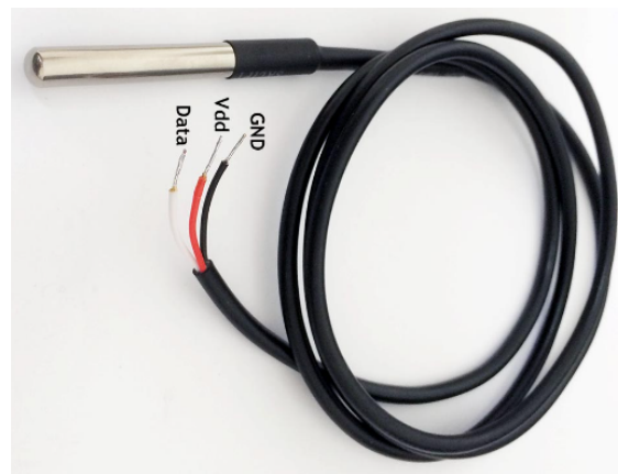
Figure 5.7: DS18B20 temperature sensor.
