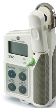
Picture 3. Chlorophyll Meter SPAD-502Plus, Konica Minolta Sensing, Inc., Japan.
