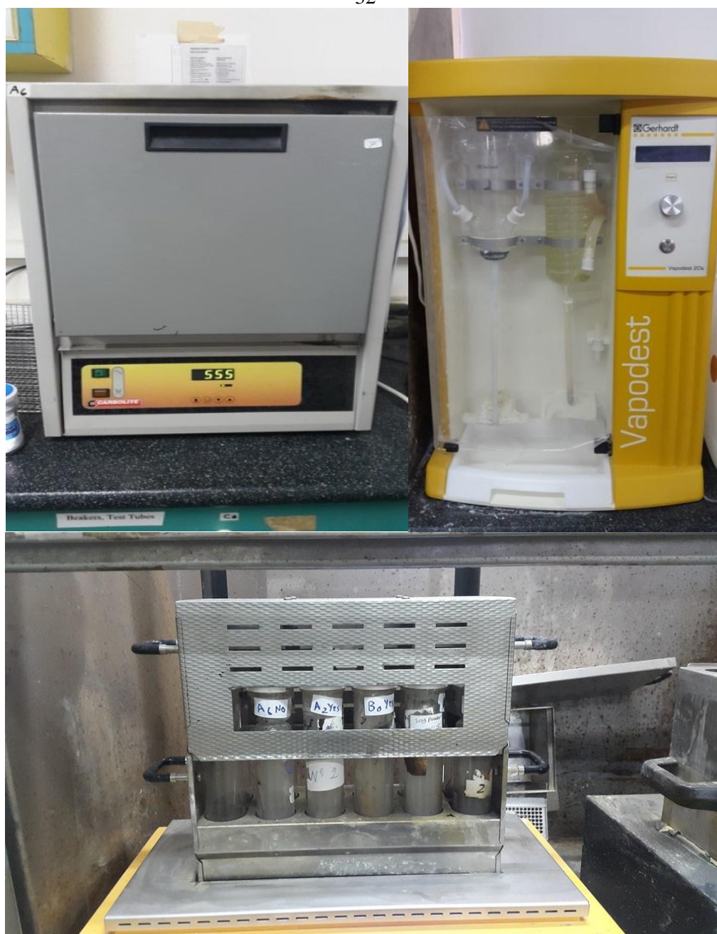
Picture 4: Carbolite (ashing samples), Turbotherm (digestion), Vapodest (Distillation).
