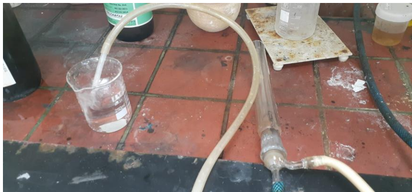
Figure (2.6): Photo of fast cooling process for Pyrex cylinder.
