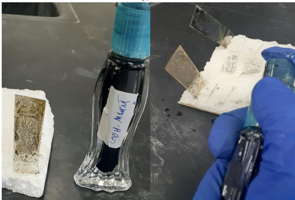
Figure (2.7): Coating process of CdS film with MWCNT
