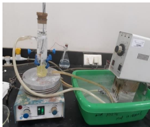
Figure (2.1): Experimental setup for solution growth of CdS film through the CBD technique
