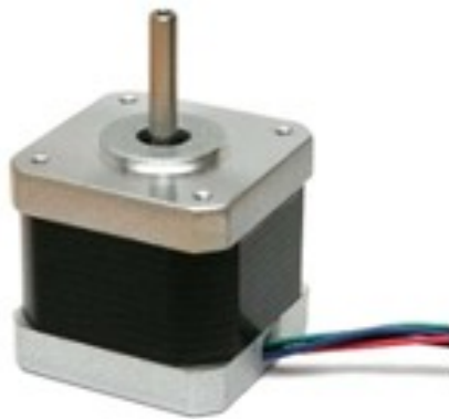
Figure 8: 12V NEMA17 stepper motor.
