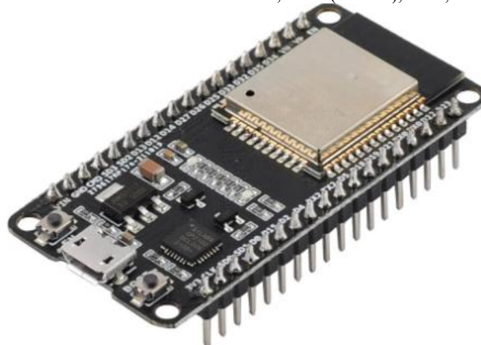
Figure 4.2: ESP32-DevKitC ESP32-WROOM-32U Core Board
