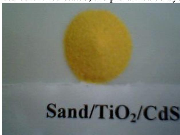
**Figure 2.5:** The visual inspection of prepared Sand/TiO<sub>2</sub>/CdS catalyst.
