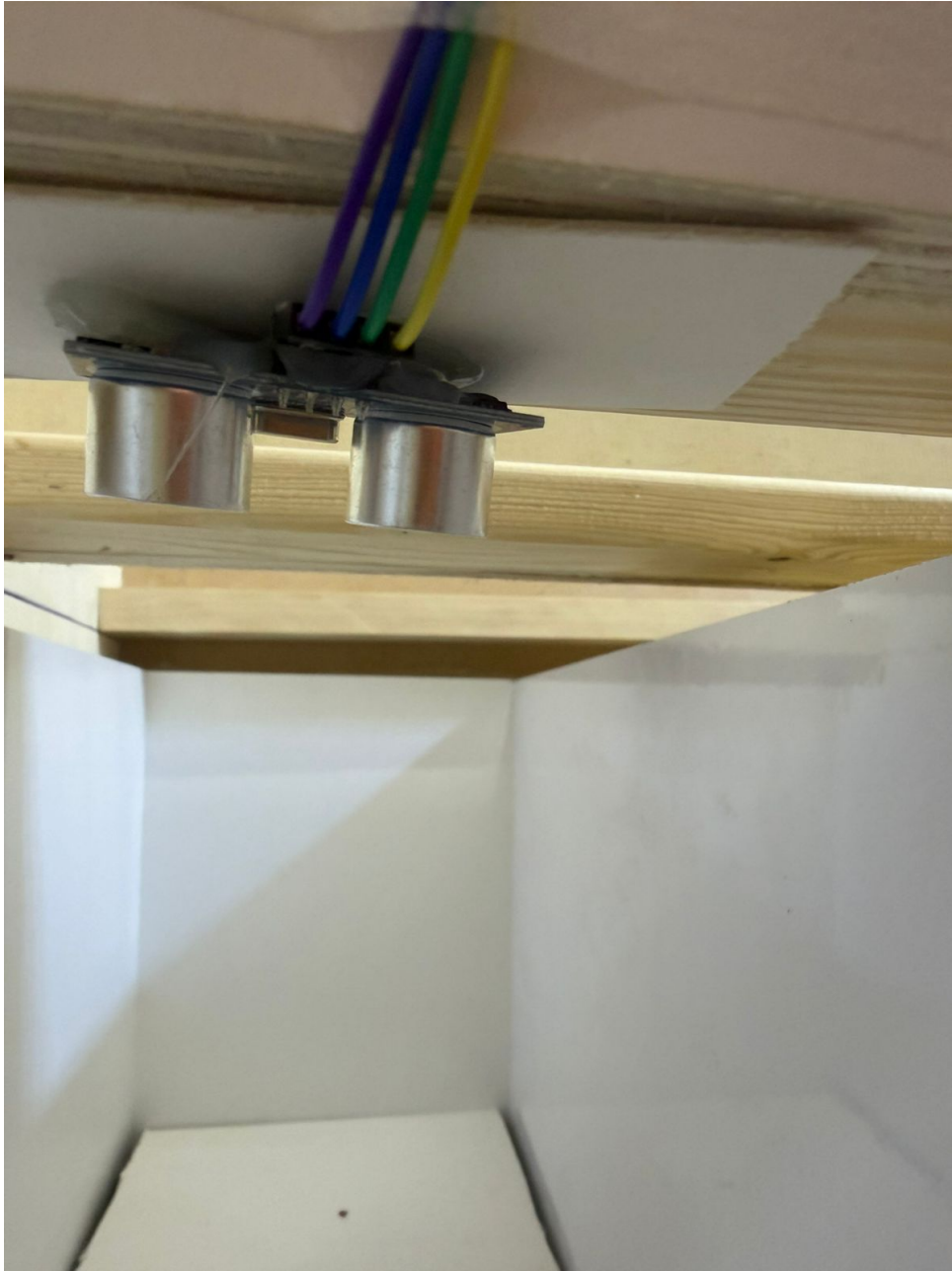
Figure 3.12: Ultrasonic sensors used for bin fullness detection.
