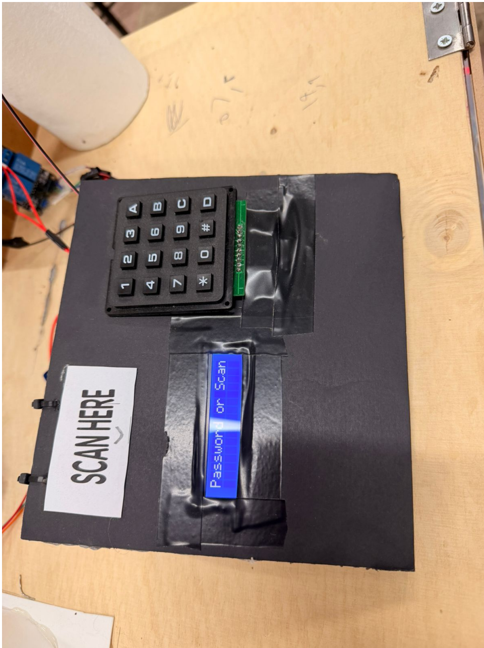
Figure 3.14: Main control panel display with keypad and RFID module.
