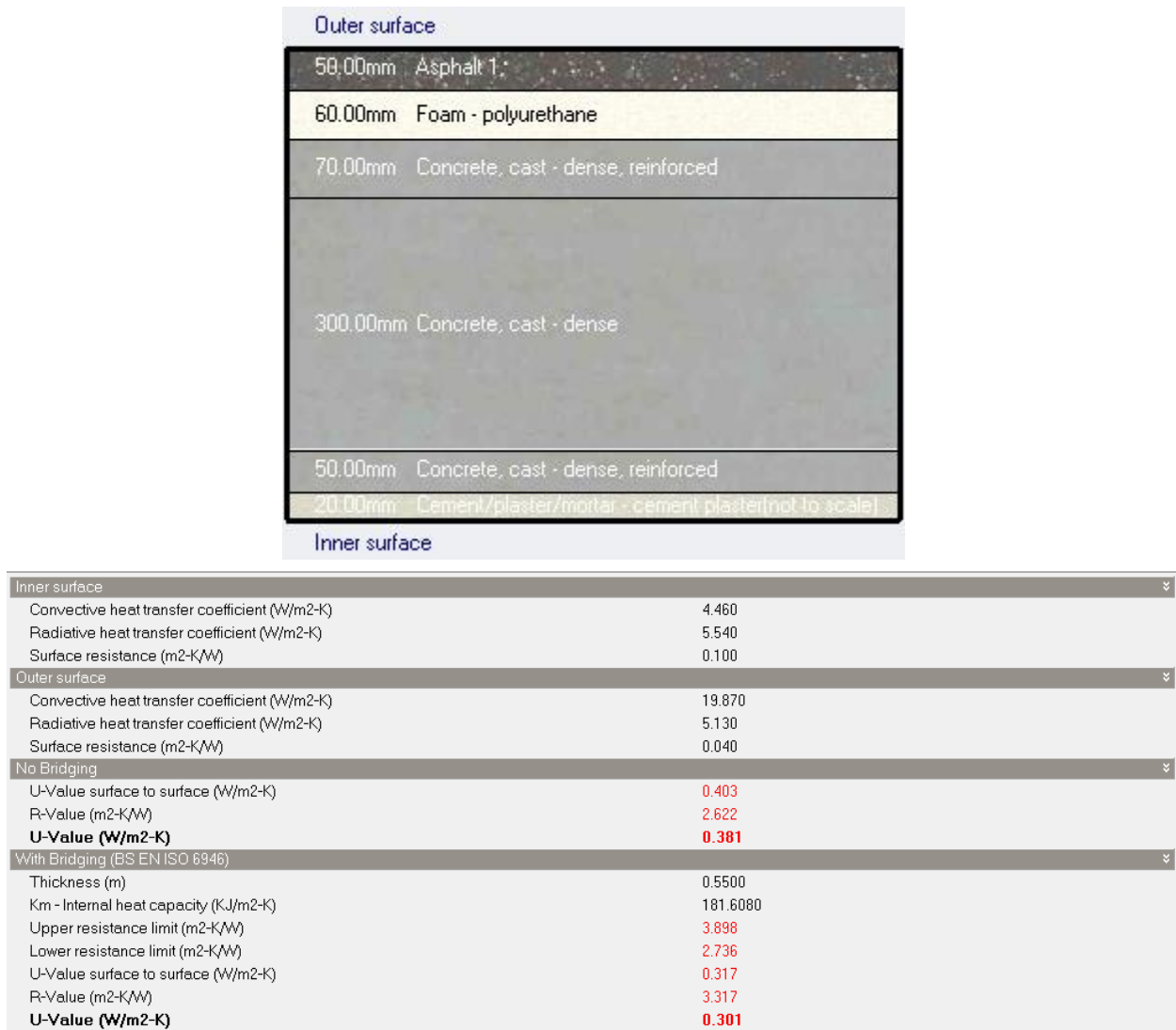
Figure 247 material properties of roof layers.
