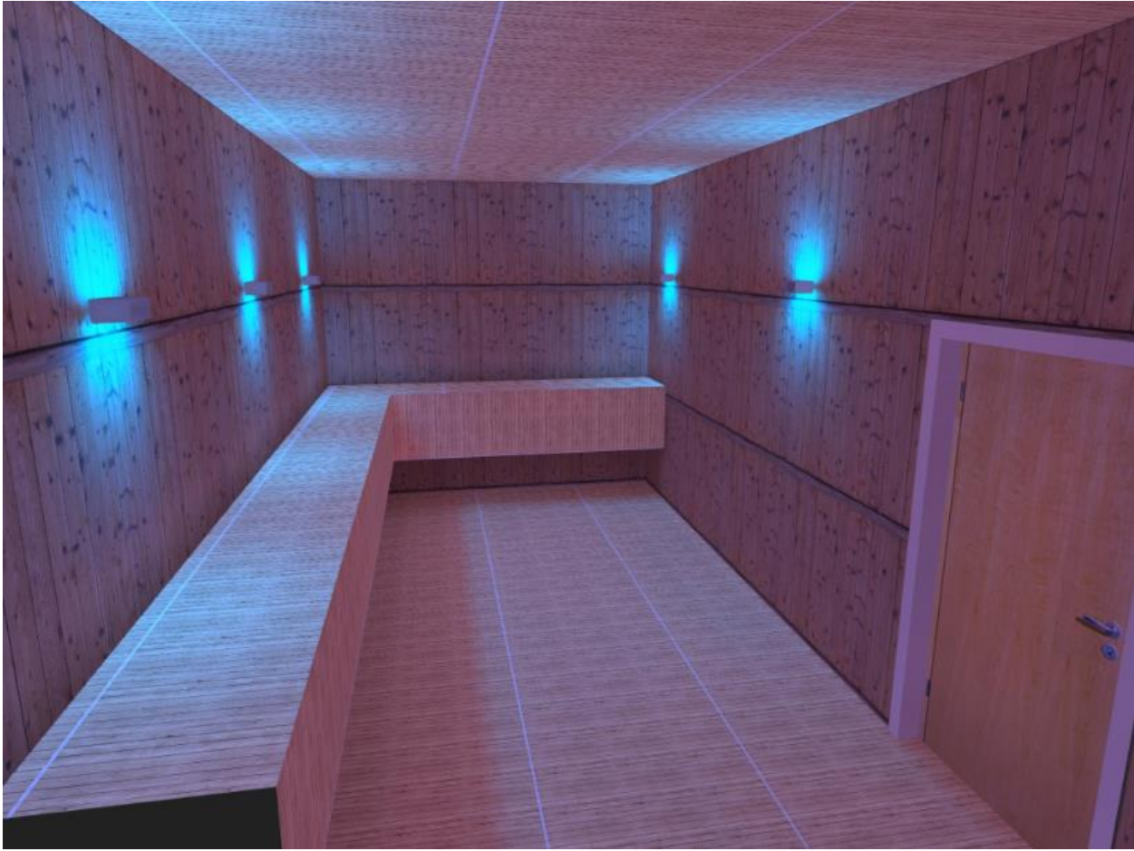
Figure 195 Steam room lighting from dialux
