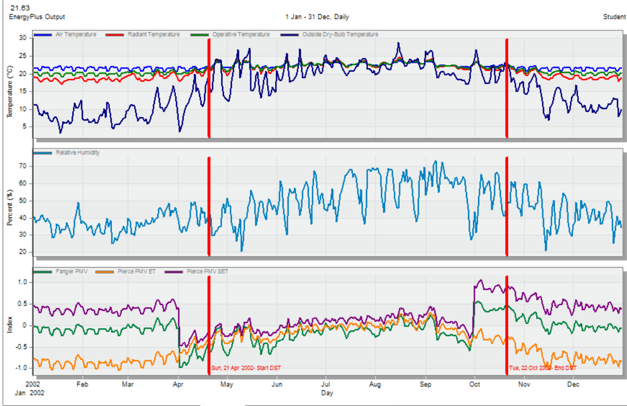
Figure 259 design builder result without using insulation
