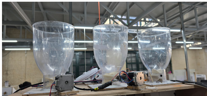
Figure 4.3: Ingredient Dispensers driven by NEMA 17 Steppers
