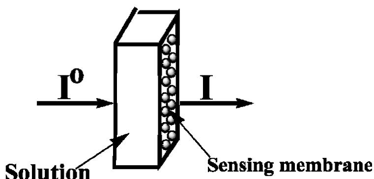
Figure 2.1: Diagram of optical sensing system.
