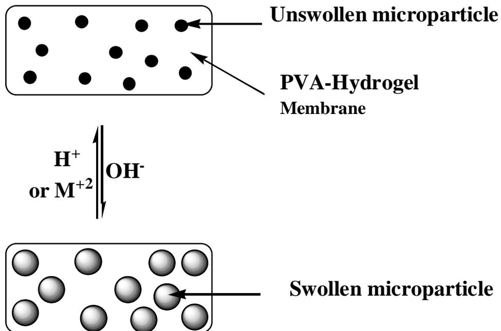
Figure 1.1: Schematic diagram of sensing response to pH and metal ions.
