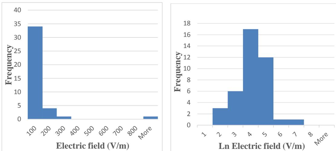
**Fig (4. 23):** A histogram of ELF electric fields (left) and ln of ELF electric fields (right) based on maximum recorded intensities at the 40 power lines.
