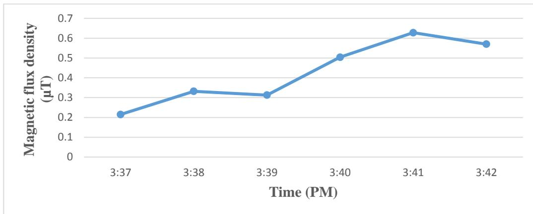
**Fig (4. 15):** Variations of background ELF magnetic flux densities over 6-minutes period, and one meter above ground level at residence R5.
