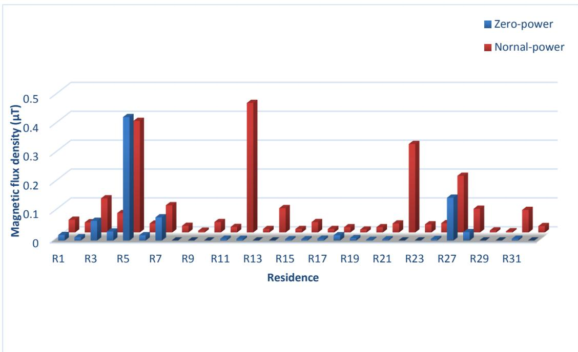
**Fig (4. 20):** Comparison of average ELF magnetic flux densities under zero and normal-power uses.
