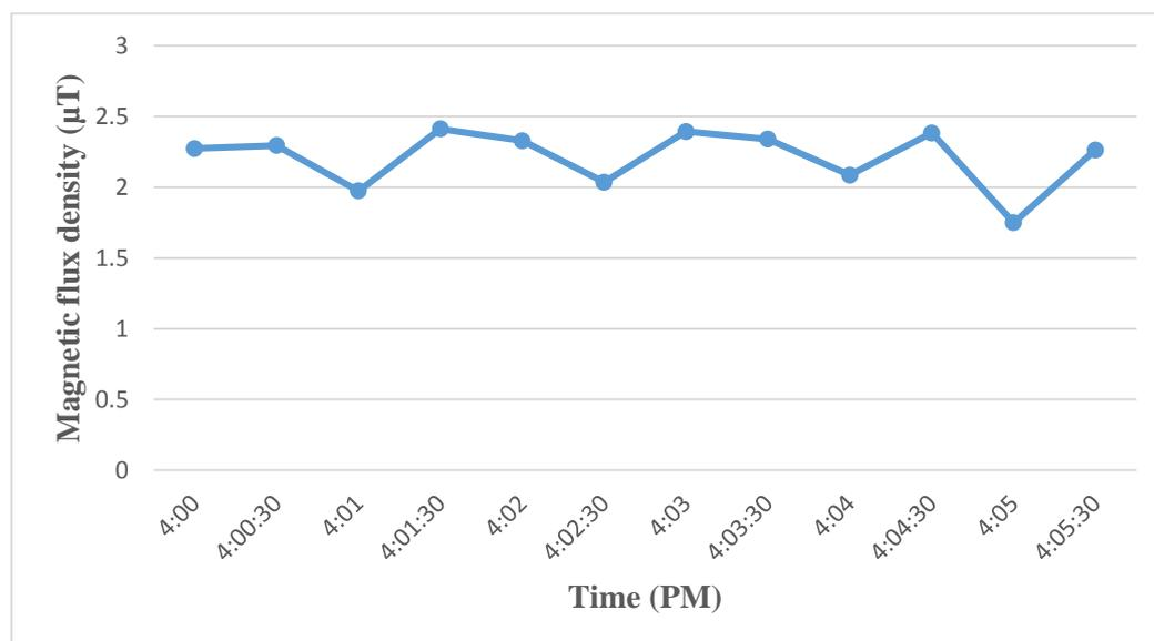
**Fig (4. 5):** Variations of ELF magnetic flux densities over 6-minutes period, and one meter above ground level under power line P38.
