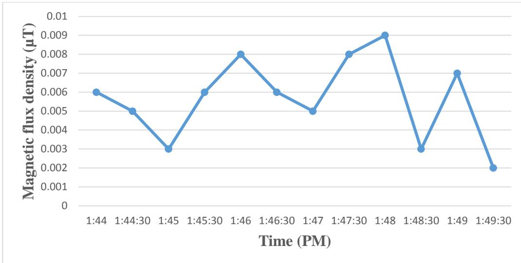
**Fig (4. 9):** Variations of ELF magnetic flux densities over 6-minutes period, and one meter above ground level at residence R9.
