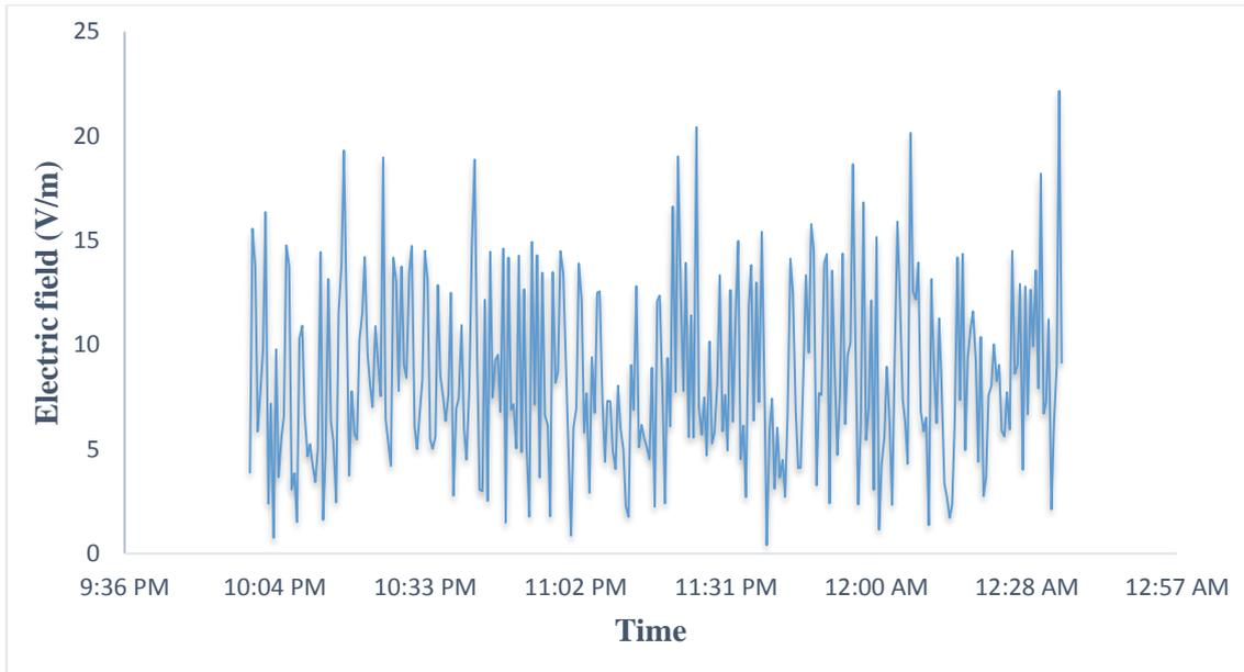
**Fig (4. 13):** Variations of ELF electric fields over 2.5 hours period, and one meter above ground level at residence R10.
