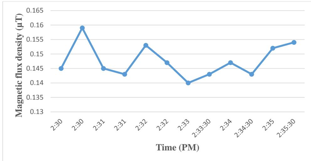
**Fig (4. 17):** Variations of background ELF magnetic flux densities over 6-minutes period, and one meter above ground level at residence R27.
