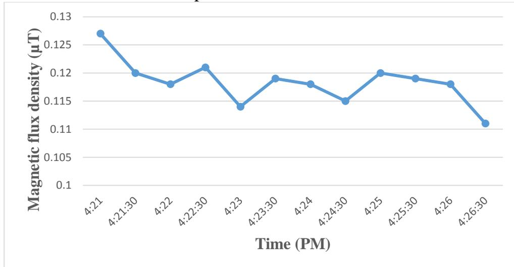
**Fig (4. 7):** Variations of ELF magnetic flux densities over 6-minutes period, and one meter above ground level at residence R3.
