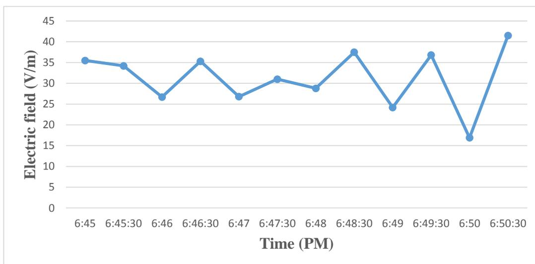
**Fig (4. 12):** Variations of ELF electric fields over 6-minutes period, and one meter above ground level at residence R12.
