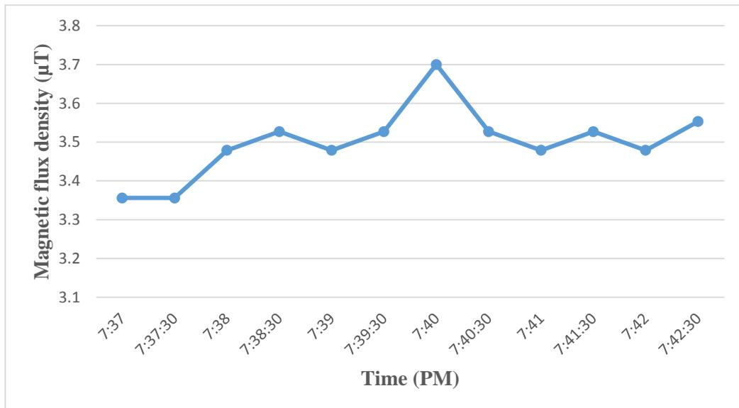
**Fig (4. 3):** Variations of ELF magnetic flux densities over 6-minutes period, and one meter above ground level under power line P33.
