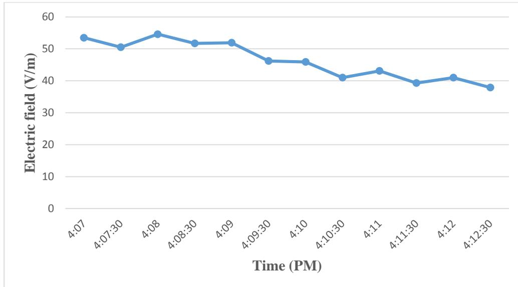
**Fig (4. 6):** Variations of ELF electric fields over 6-minutes period, and one meter above ground level under power line P38.
