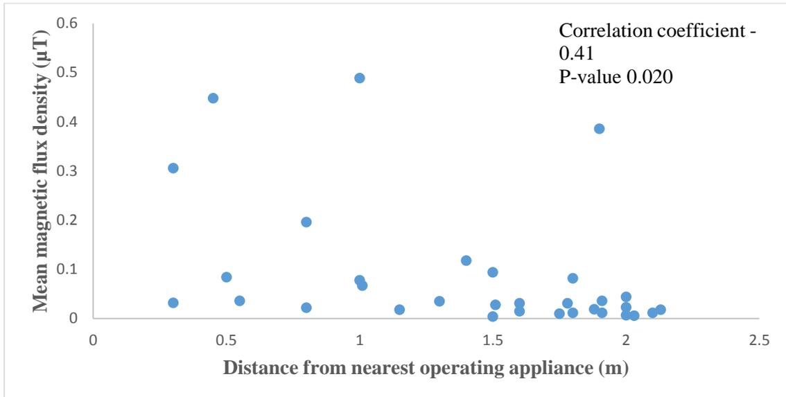
**Fig (4. 30):** A scatter plot showing the moderate negative correlation between mean magnetic fields measured among the 32 residences and distance from nearest operating appliance.
