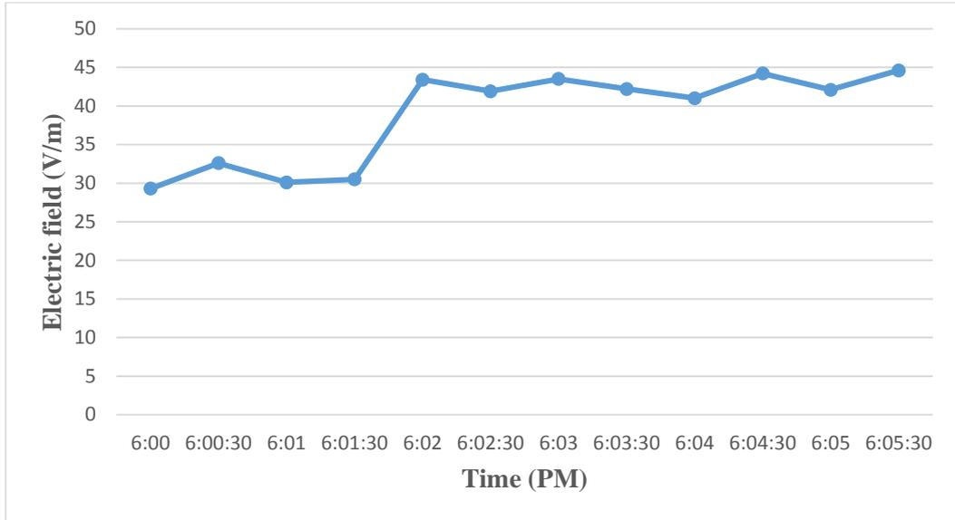
**Fig (4. 2):** Variations of ELF electric fields over 6-minutes period, and one meter above ground level under power line P8.
