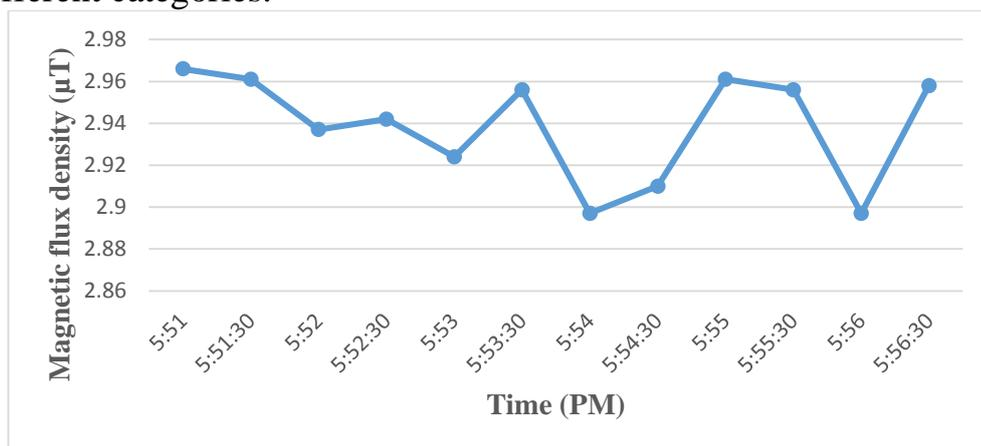
**Fig (4. 1):** Variations of ELF magnetic flux densities over 6-minute period, and one meter above ground level under power line P8
