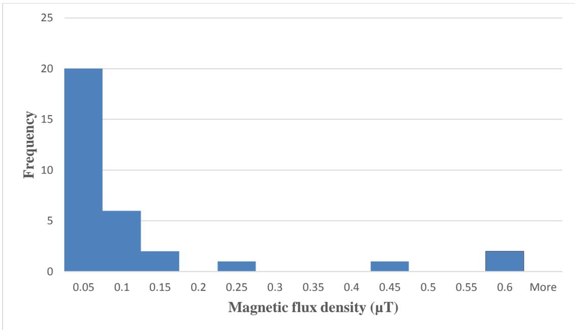
**Fig (4. 27):** A histogram of ELF magnetic flux densities based on maximum recorded fields at the 32 residences.
