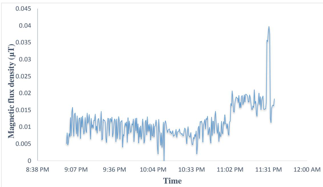
**Fig (4. 14):** Variations of ELF magnetic flux densities over 2.5 hours period, and one meter above ground level at residence R10.
