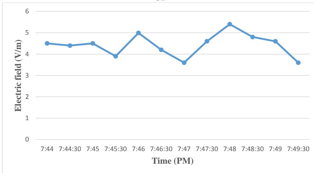
**Fig (4. 4):** Variations of ELF electric fields over 6-minutes period, and one meter above ground level under power line P33.
