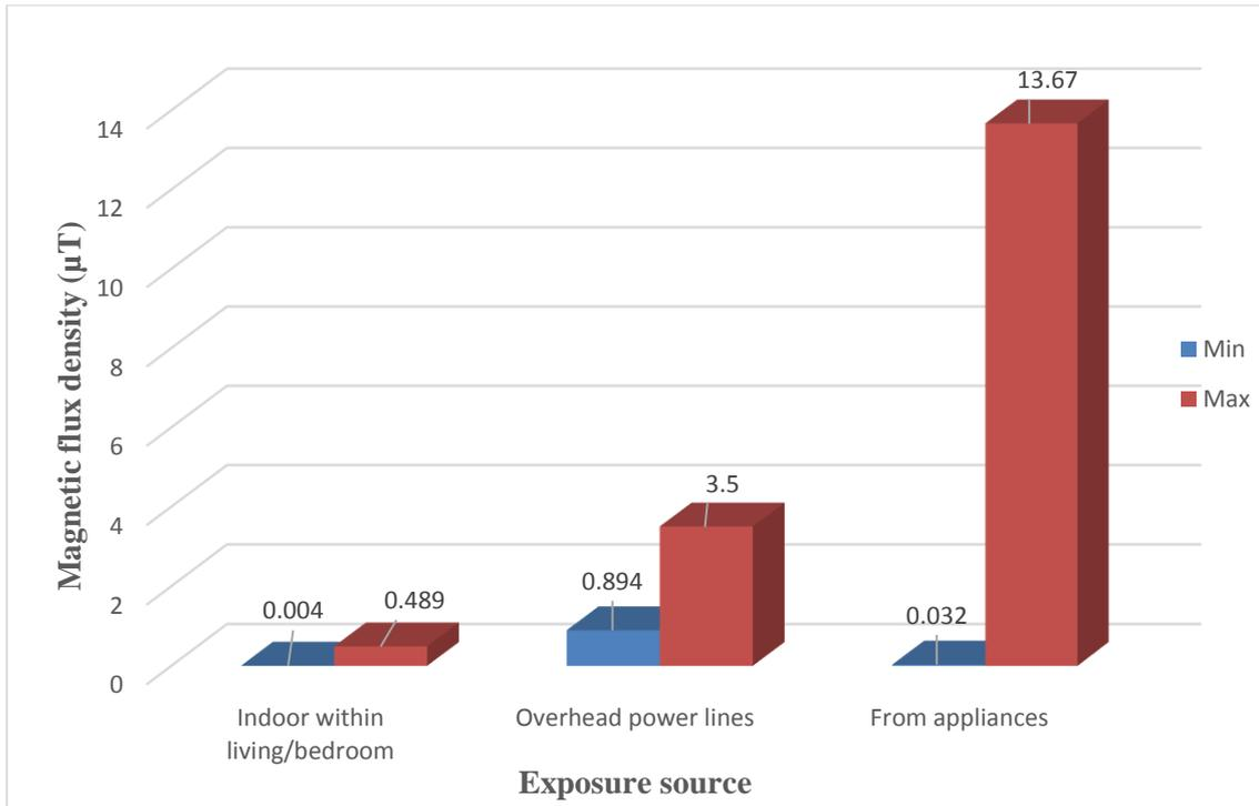
**Fig (5. 2):** Comparison of minimum and maximum exposures to ELF magnetic flux densities based on different sources.
