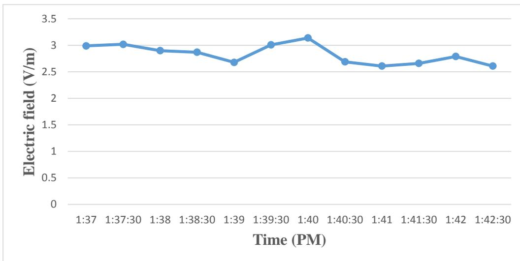
**Fig (4. 10):** Variations of ELF electric fields over 6-minutes period, and one meter above ground level at residence R9.
