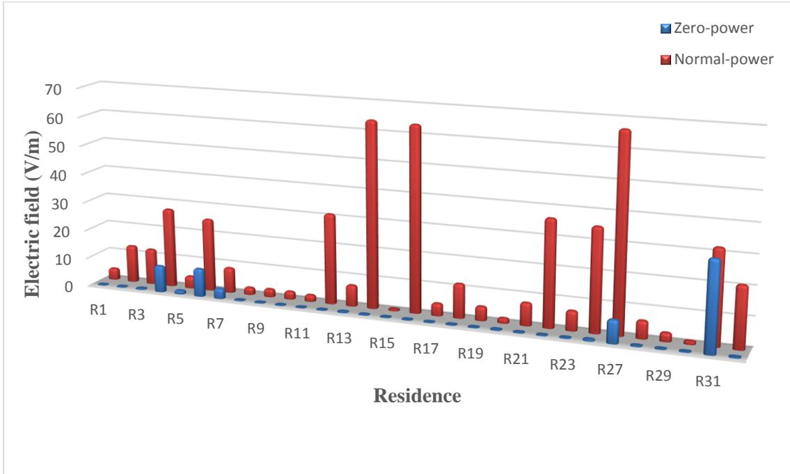
**Fig (4. 19):** Comparison of average ELF electric fields under zero and normal-power uses.
