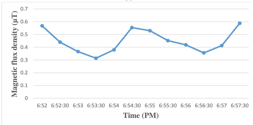
**Fig (4. 11):** Variations of ELF magnetic flux densities over 6-minutes period, and one meter above ground level at residence R12.
