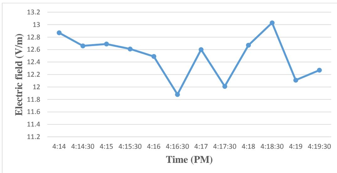
**Fig (4. 8):** Variations of ELF electric fields over 6-minutes period, and one meter above ground level at residence R3.
