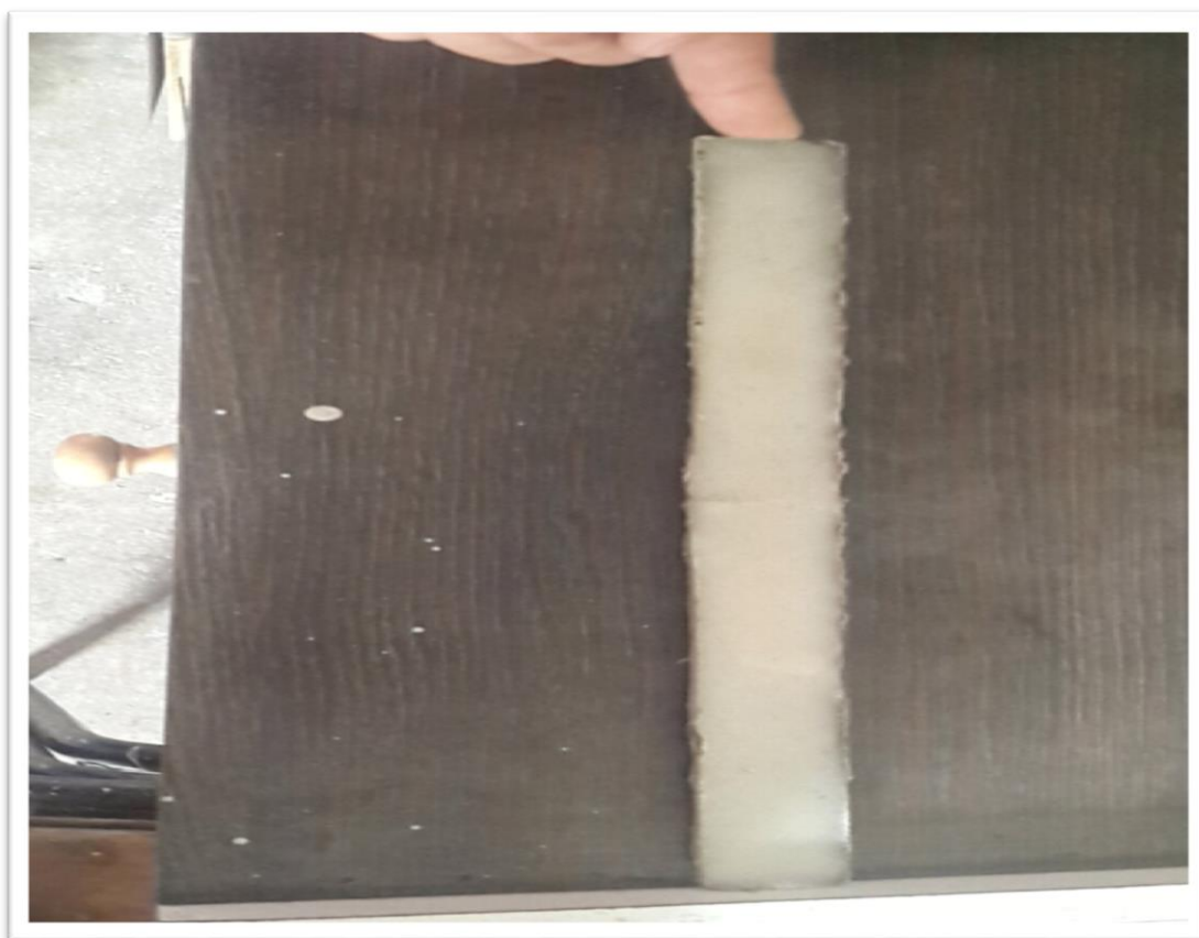
Figure 3.10: An epoxy blended with EPO sample after 24 hours tensile strength by tensile machine.
