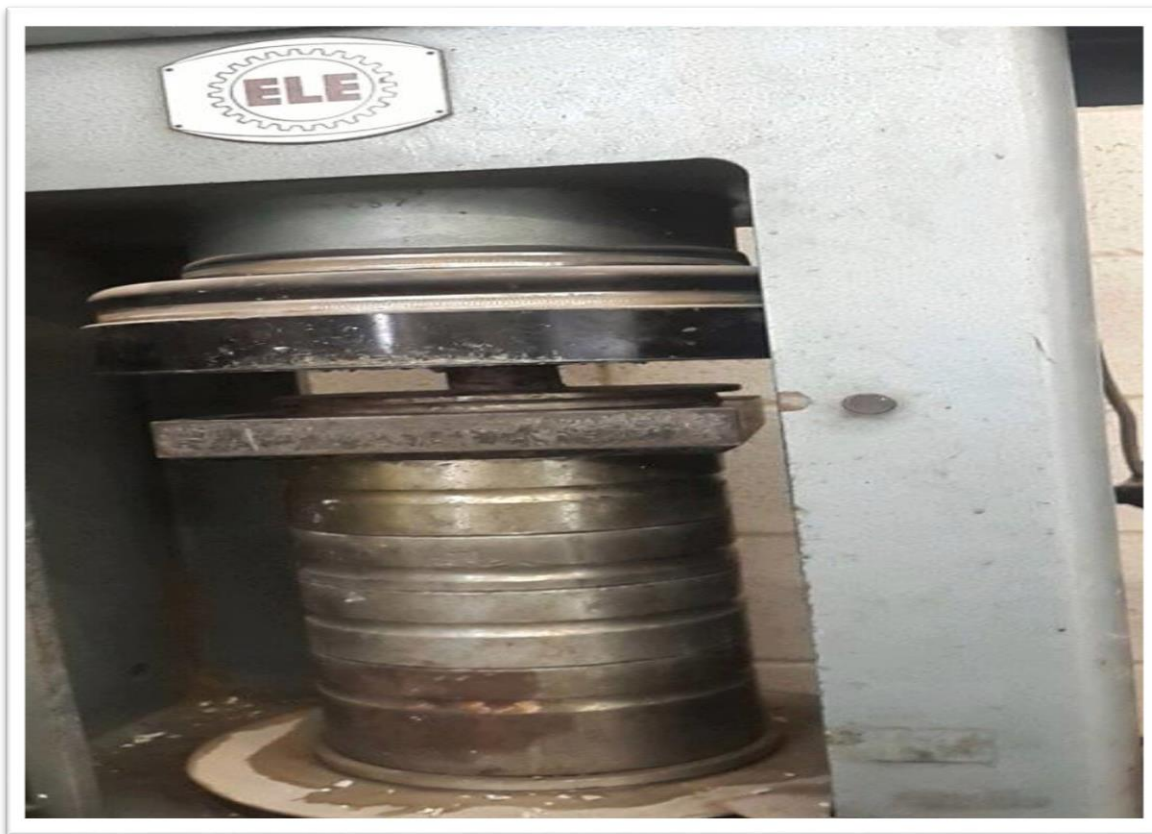
Figure 3.5: An epoxy with EPO sample after 24 hours' compression strength by compression machine.
