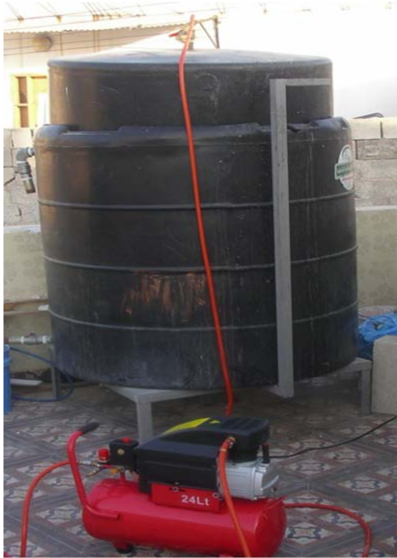
Photo 3.5: Withdrawing biogas from digester into air compressor
