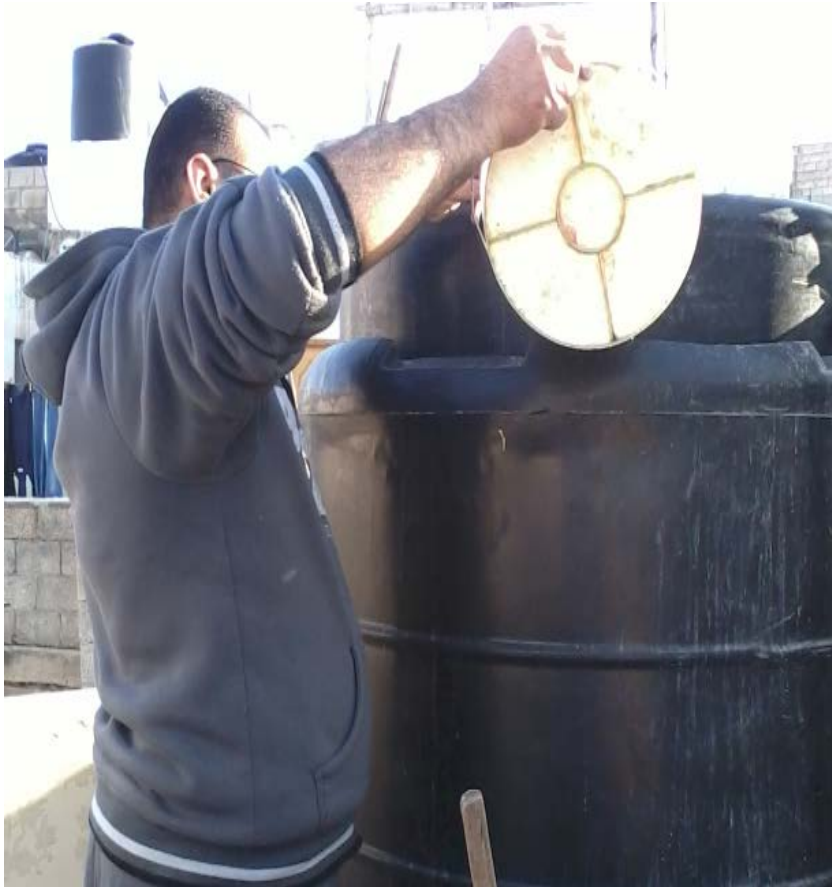
Photo 3.4: Introducing sample into the digester
