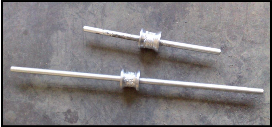
Figure 1. 3 The driving shafts each one has a pulley, the tall one is for cartage 1 and the short one is for cartage 2.
