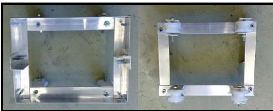
Figure 1. 5 cartage 1 parts, a) the lower track base, b) the upper track base and c) the housing of bases.
