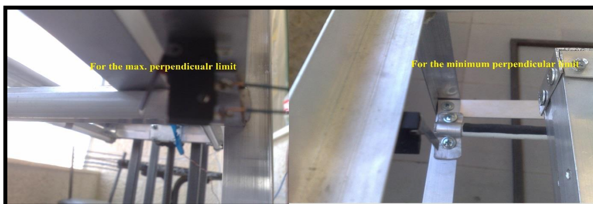
Figure 2. 15 limiting the perpendicular motion two limit switches are used
