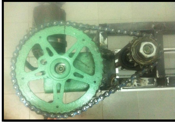
Figure 1. 10 A gear on top of the screw acquires motion from the driving gear through a chain between them.
