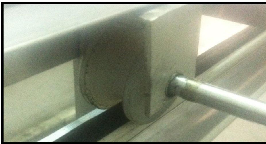
Figure 1. 2 a driving wheel type sliding over the aluminum rod track.
