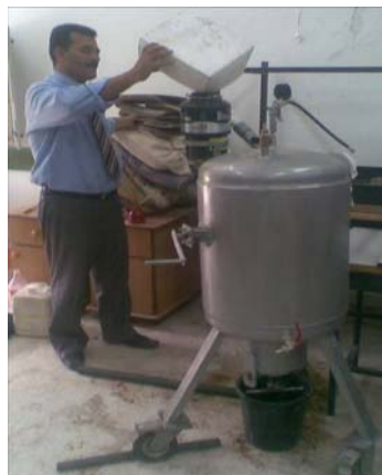
Picture (1): Nablus Industrial School Digester as Family Size Units.
