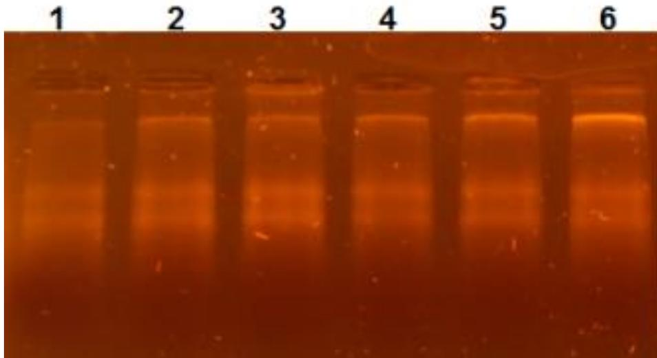
**Figure 4-3.** Example of electrophoresis of total RNA extraction. 1.2% agarose gel in TBE, colored with GelRed (Biotium). Lane 1-6 represents TNA from different fig leaf samples.
