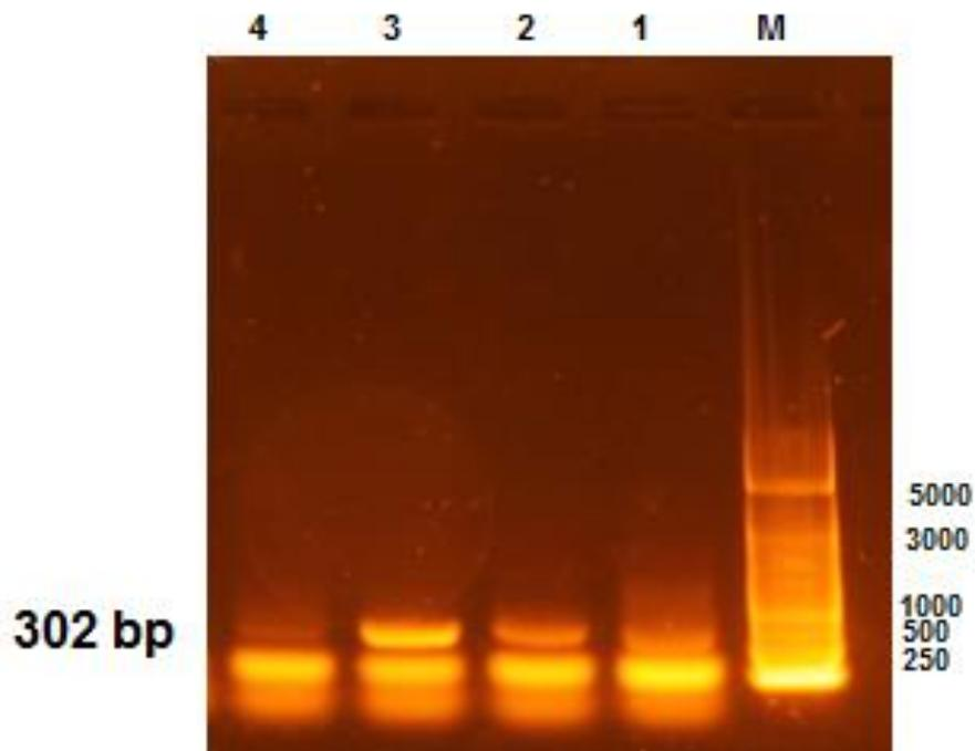
**Figure 4-4.** PCR results of FMV: Lane **M** contained ladder (1Kb DNA ladder RTU, GeneDireX)), lane **4** represents negative sample, lane **1, 2 and 3** represents FMV positive sample on 302 bp.
