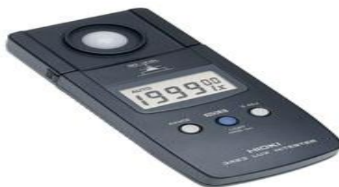
Fig. 3.2 Hioki 3423 Lux Hitester Digital Illumination Meter (Instruction Manual for Lux Hitester, Japan, 2006)
