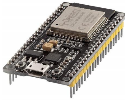
Figure 3: ESP32 Module - provides Bluetooth connectivity for mobile app
