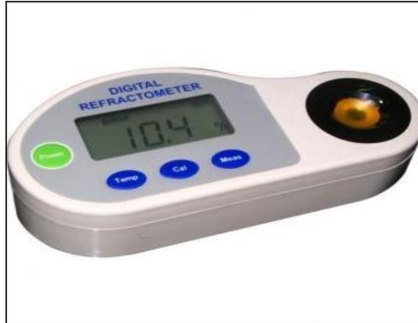
**Fig.(3.4):** Digital Refractometer
