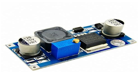
Figure 3.17: LM2596 DC-DC buck converter
