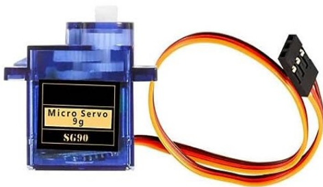
Figure 3.9: SG90 servo motor.
